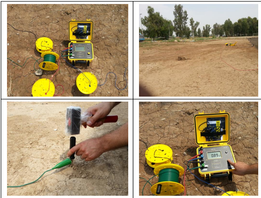
Figure (4-6) soil resistivity measurements
