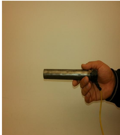
Figure (4-2) scrap steel Anode
