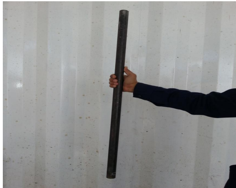
Figure (4-1) carbon steel pipe (cathode)
