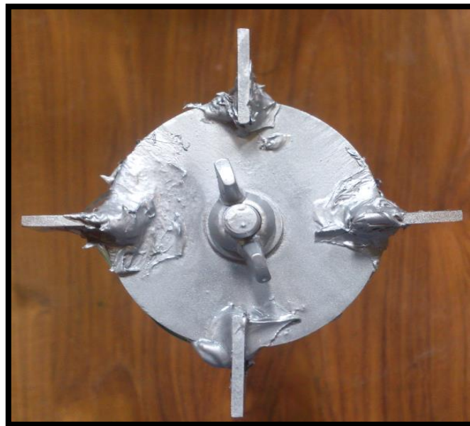
Figure 3-2 Circular Disk Turbine (four- blades).
