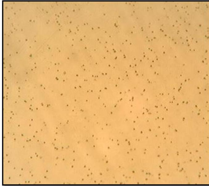
**Figure 3-41** First step from image processing of Image-J program which obtained the track image in CN-85 detector after 24h irradiated time -  $T_D$
