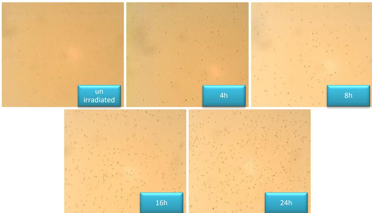
**Figure 3-1** Images by optical microscope of CR-39 detector irradiated with thermal neutrons for different irradiation times ( un-irradiated, 4h, 8h, 16h and 24h)
