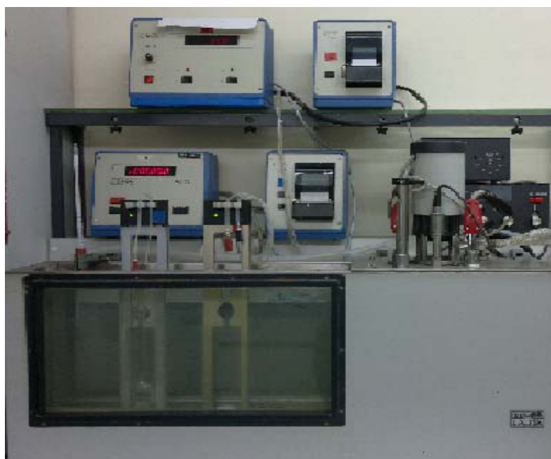
Figure 3-3 Water Bath with Viscometer.
