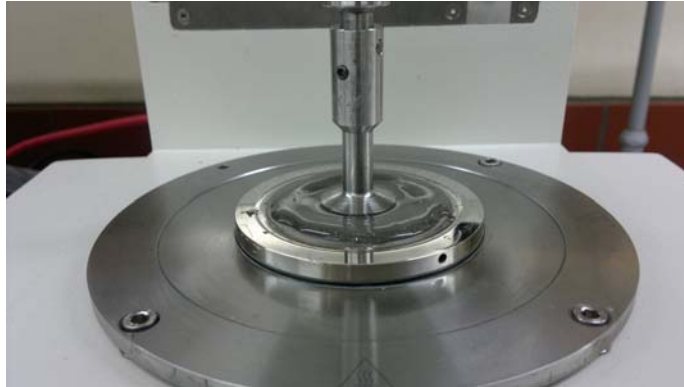
Figure 3-6 Set up of cone/plat measurements
