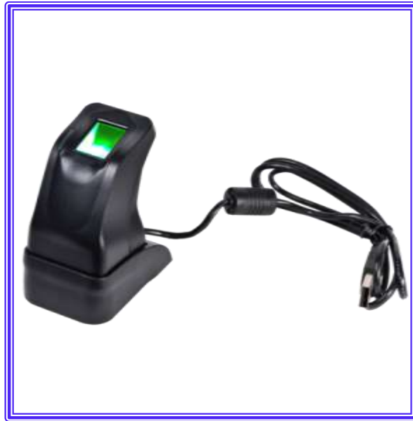
Figure 4-2: ZK 4500 FP scanner
