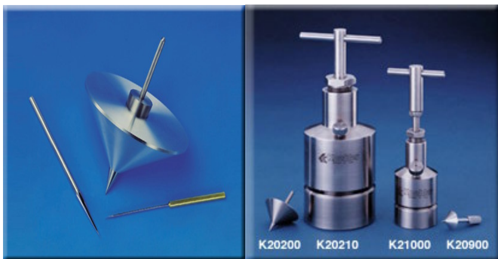
Fig. 3.4: Apparatus hammer used for penetration measurements
