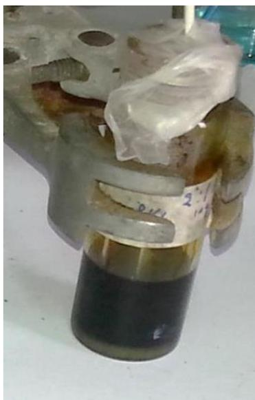
*Figure (3-2): Optical photograph for ionic liquid 2:1 mole ratio diluted with 35v% of toluene.*
