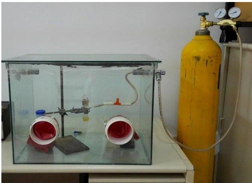
*Figure (2-1): The glove box under nitrogen gas.*
