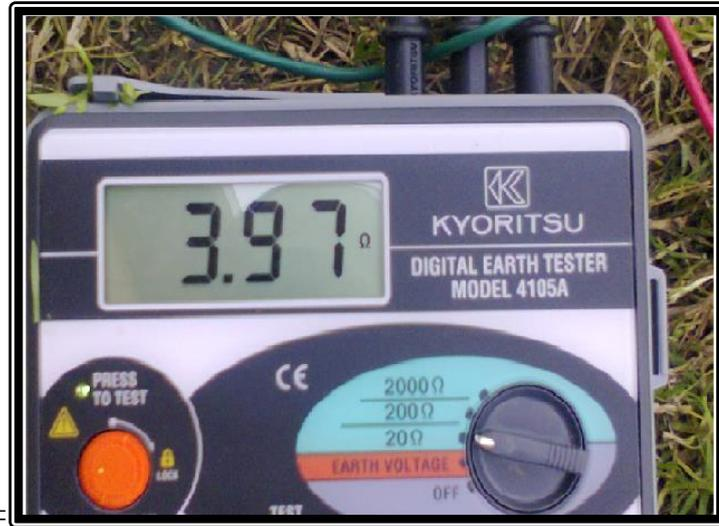
*Figure 2.9: Earth tester reading.*
