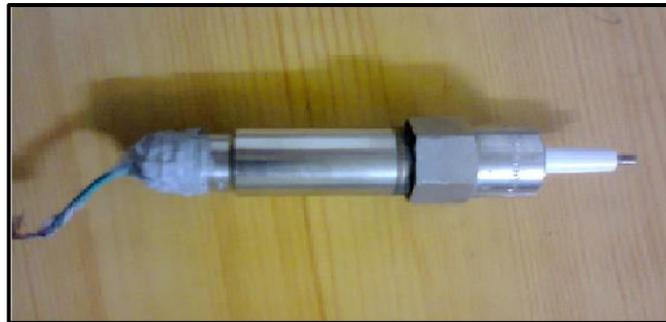
*Figure 2.1: Plug of trigger unit*
