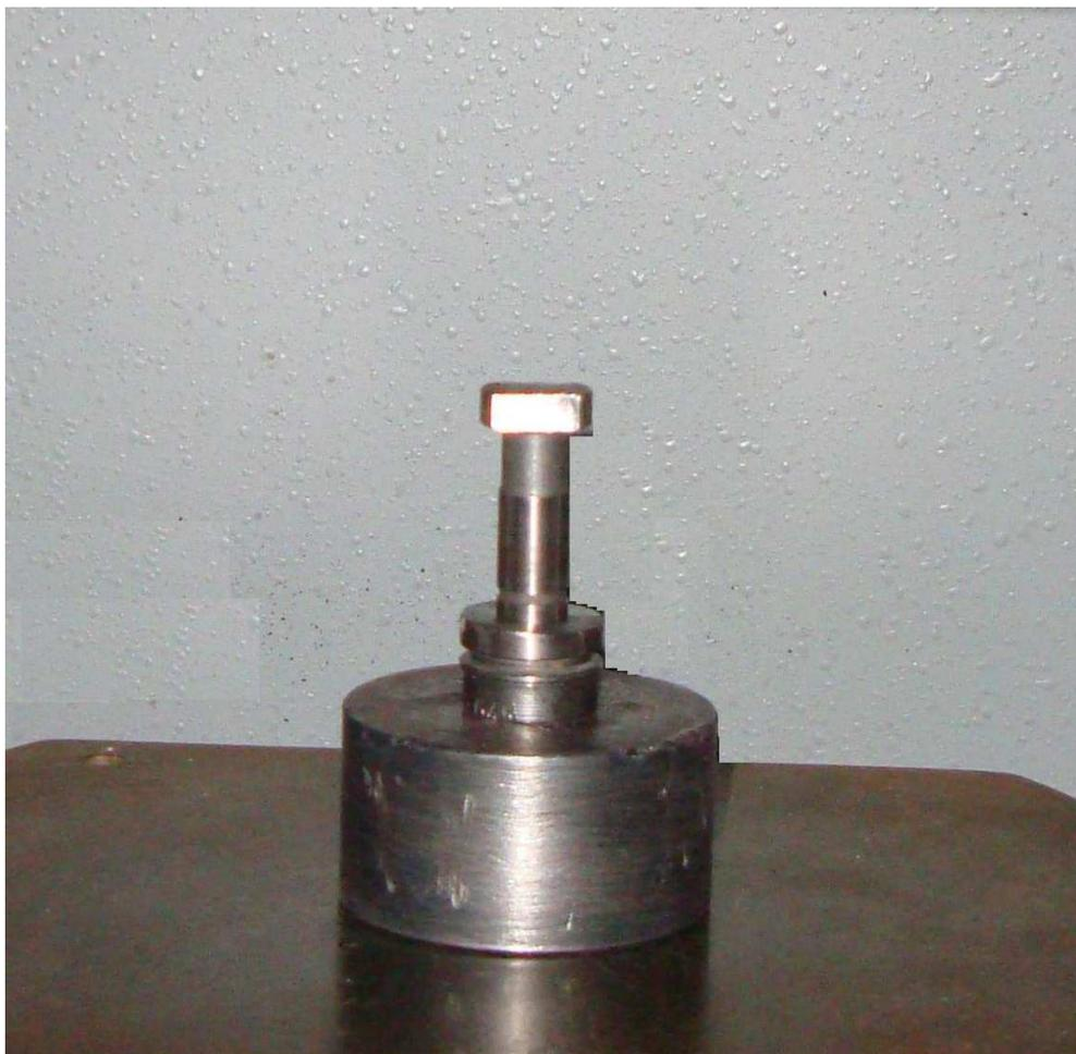
Fig. 2.5: The template used for pressing the powders.
