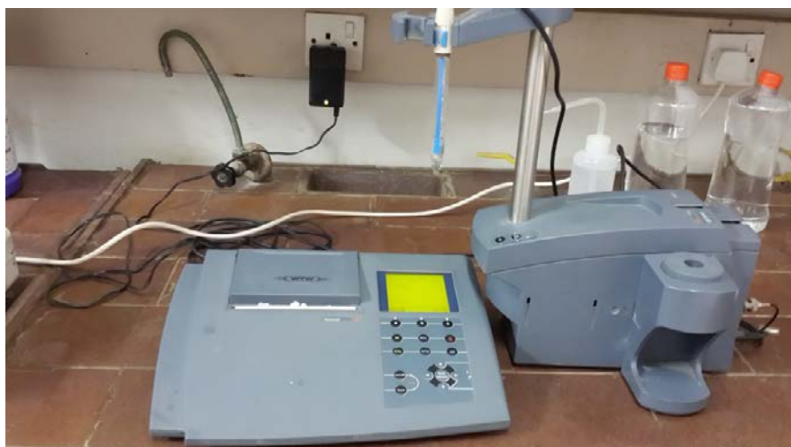
Figure 2-1:- A digital pH/ion meter (inoLab 740 with terminal 740 – WTW,
