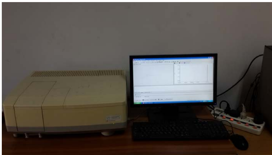
Figure 2-2:- Double-beam UV-Visible spectrophotometer model (UV-1650 PC) SHIMADZO(Japan).
