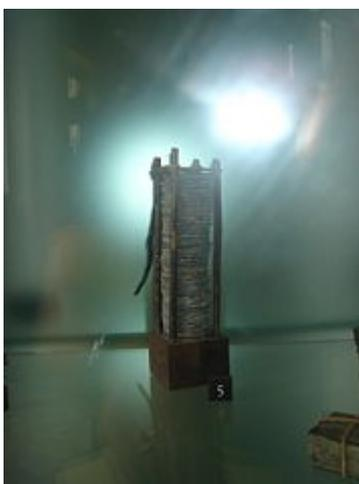
**A Voltaic Pile, the first modern battery.**
