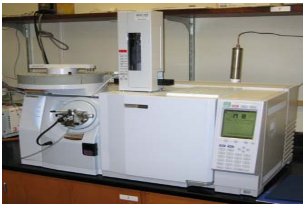
Figure (2-2): Gas Chromatograph Mass Spectrometer (GC/Mass) apparatus
