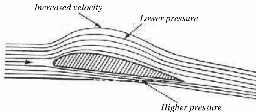
Fig (2.8) Pressure created by a wing in flight.
