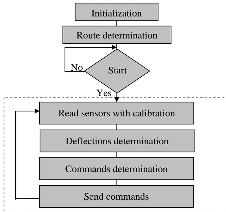
Fig (3.1) Block diagram of the auto-navigation operations.
