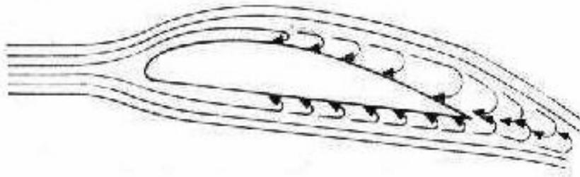
Fig (2.11) Development of the boundary layer as a result of skin friction
