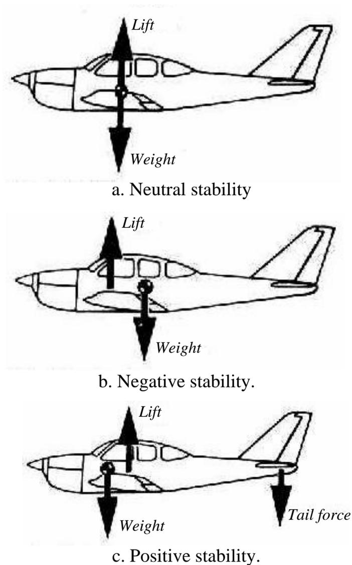
Fig (2.17) Types of airplane horizontal stability.
