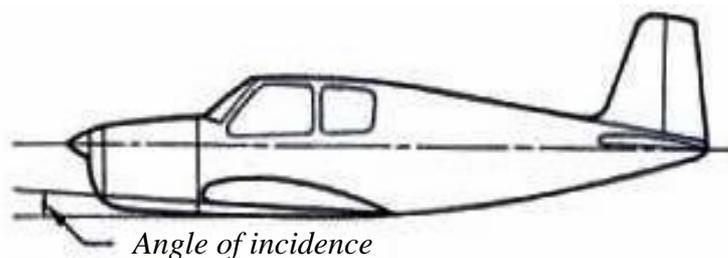
Fig (2.6) Angle of incidence.
