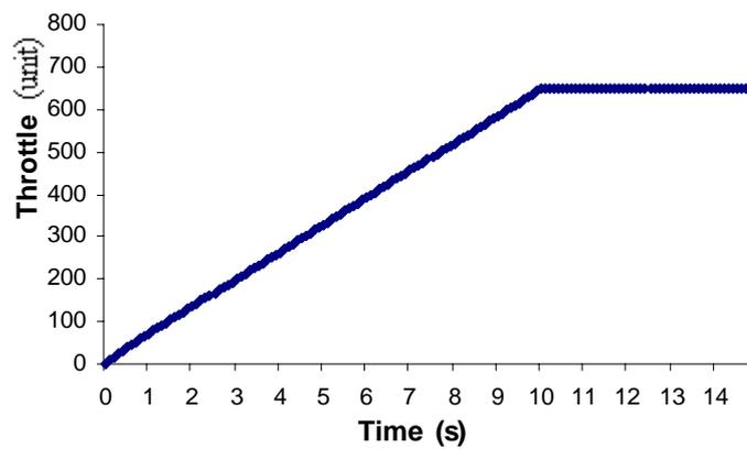
b. Throttle behavior for inefficient engine.
