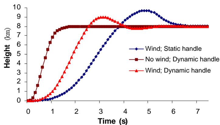
Fig (4.53) The effect of the opposite wind and static/dynamic handle on the behavior of simulated height.
