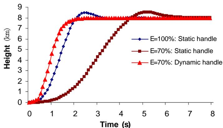
Fig (4.54) The effect of low engine efficiency and static/dynamic handle on the behavior of simulated height.
