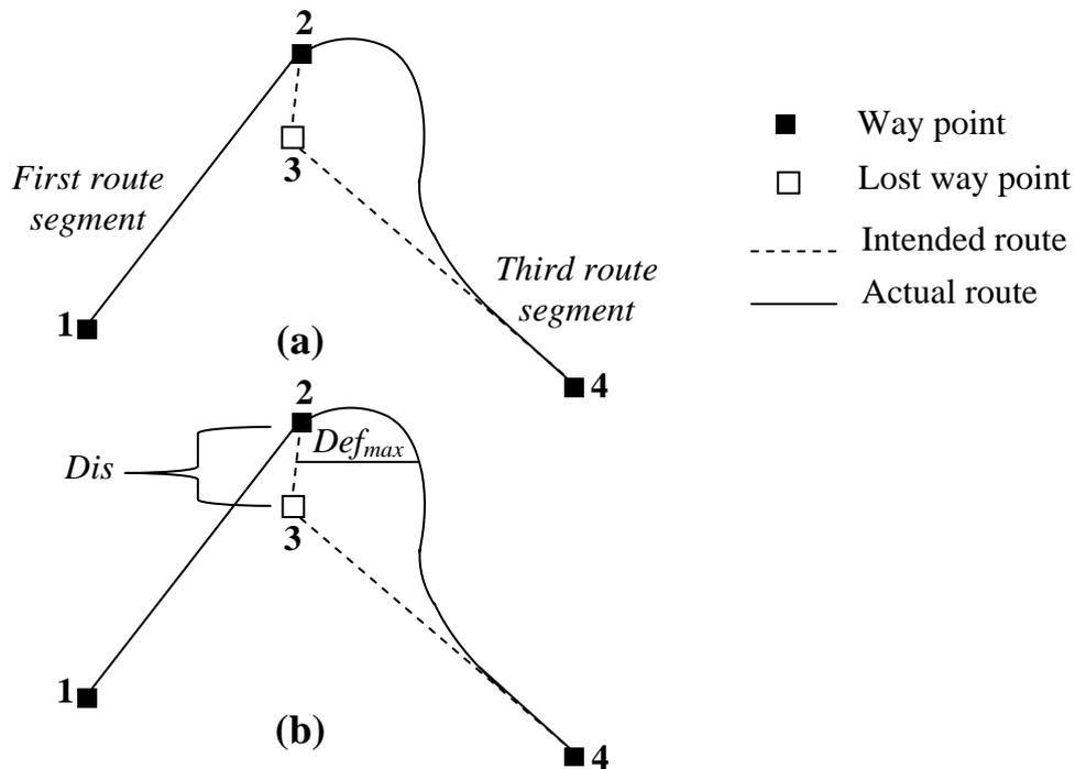
Fig (3.11) Lost way point in the intended route during a turn.
