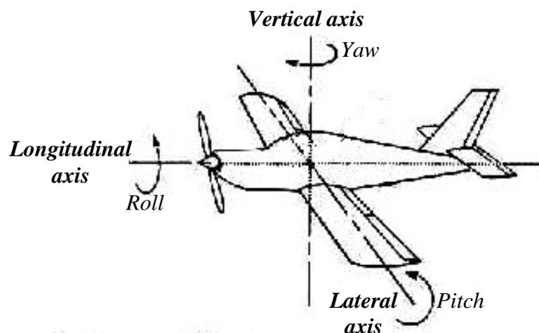
Fig (2.15) Axes of the airplane.
