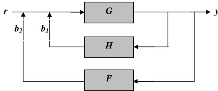
Fig (1.4) Feedback system with two feeding loops.
