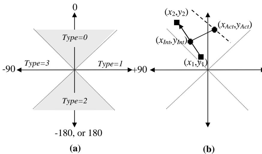
Fig (3.9) The classified four regions used in heading correction.
