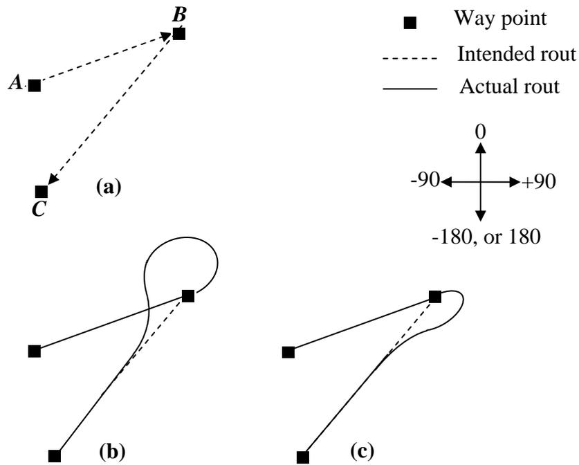
Fig (3.8) The possible turnings of an airplane.
