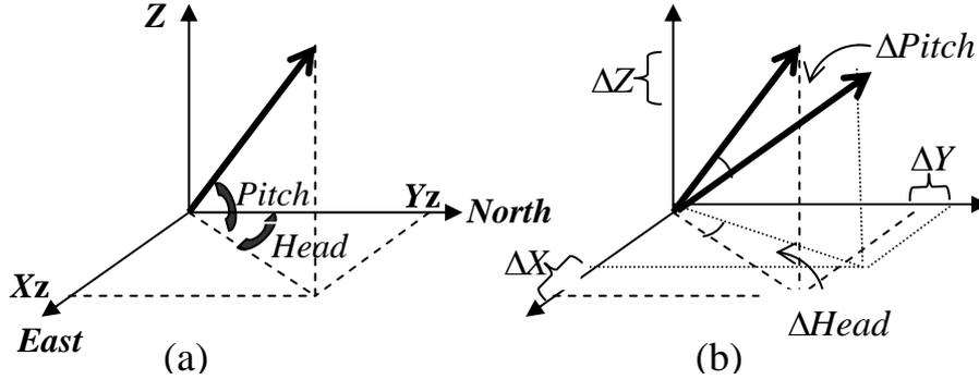
Fig (3.2) The three positioning coordinates of the airplane
