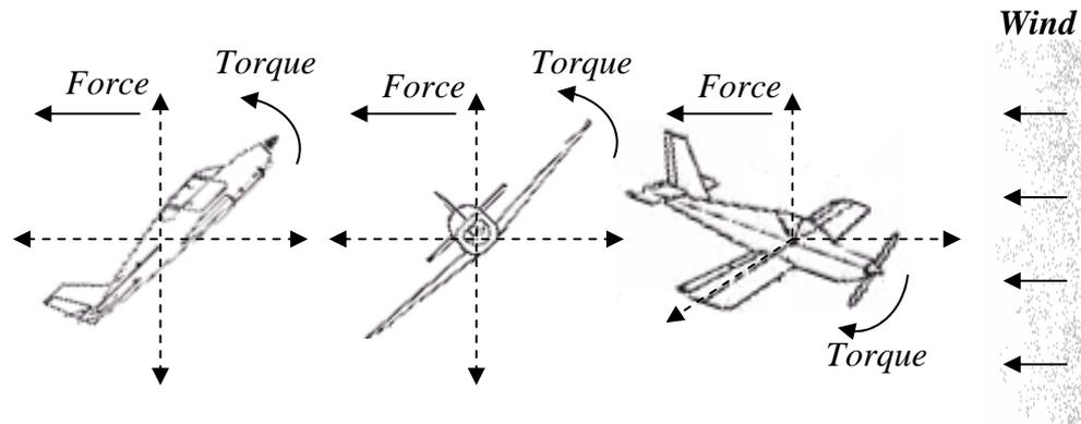
Fig (3.16) Aerodynamic forces and torques applied on the airplane by the wind.
