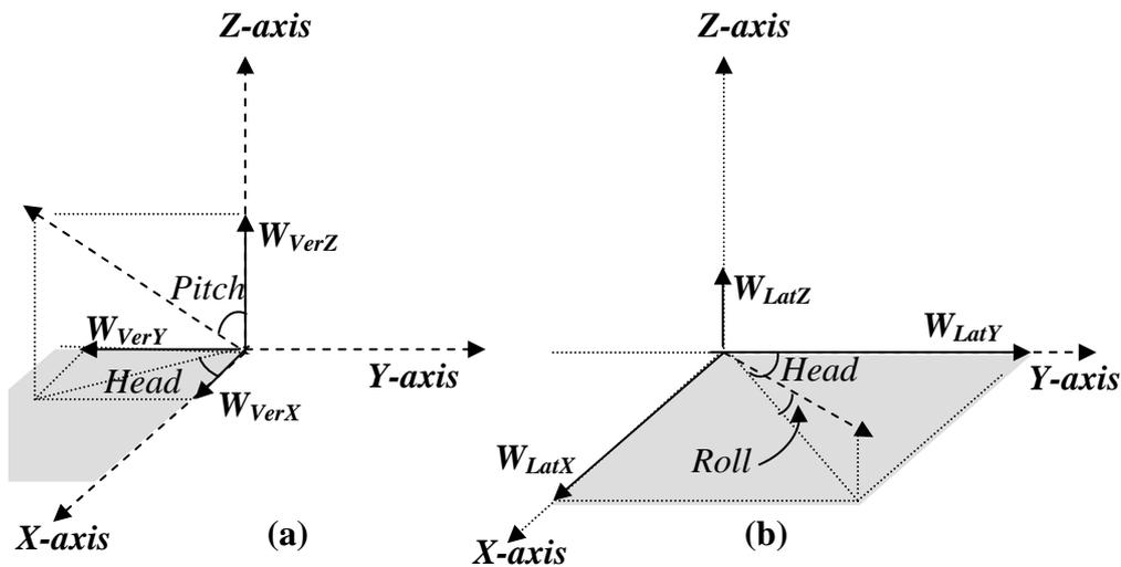
Fig (3.19) Wind speed components with respect to the reference coordinates X, Y, and Z.
