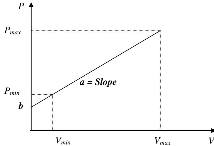
Fig (3.7) The linear relationship between the sensor's voltage output and the measured parameter value.
