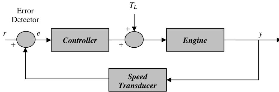
Fig (1.2) Elements of close loop control system
