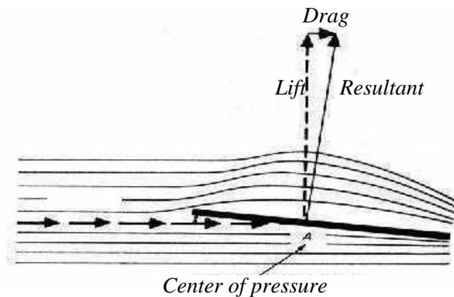
Fig (2.10) Flat plate in a stream of air
