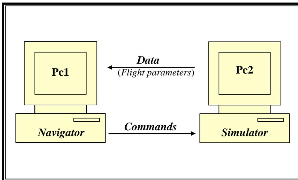
Fig (4.1) Data exchange between the navigator and simulator computers.
