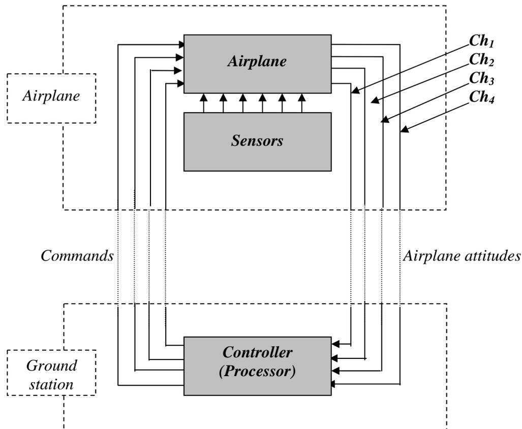
Fig (1.7) Digital auto-pilot system for a guided airplane.
