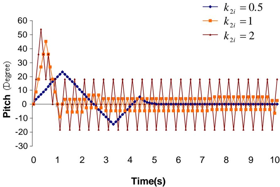
Fig (4.13) Simulated actual pitch behavior for different values of  $k_{2i}$ .
