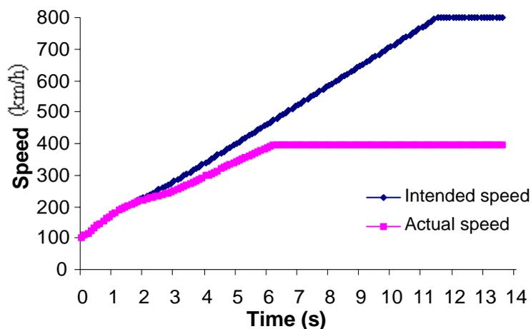
Fig (4.52) The behavior of simulated speed when both the actual speed and height are changed together, in comparison with the case of fixed height.
