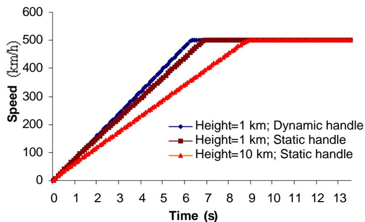
Fig (4.55) The effect of high altitude and static/dynamic handle on the behavior of simulated speed.
