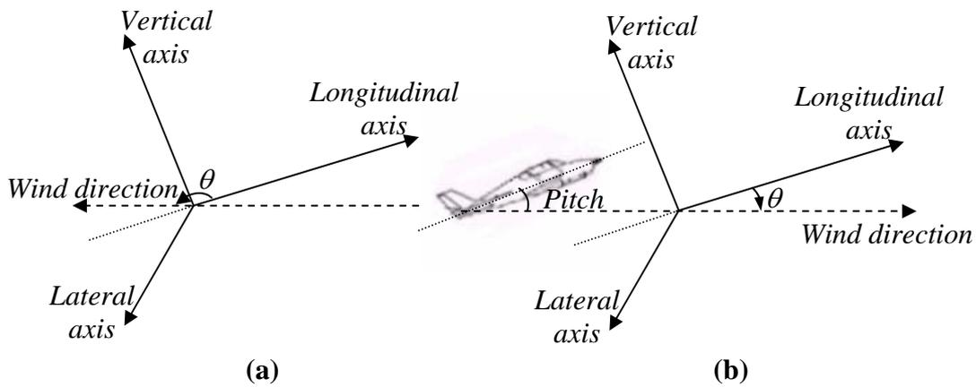
Fig (3.18) Determination of angle  $\theta$ .
