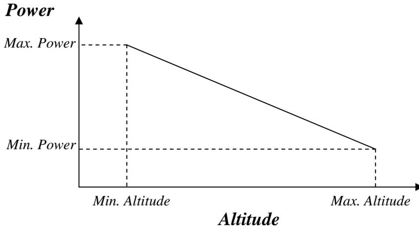
Fig (3.21) The relative engine power chart of the airplane versus altitude.
