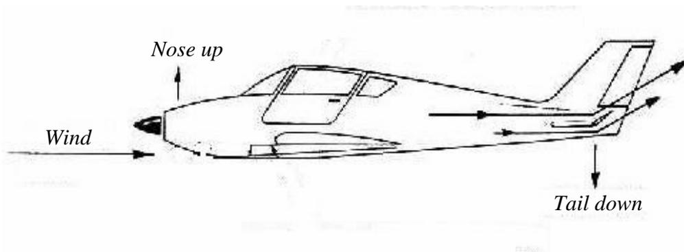
Fig (2.19) Action of elevator.
