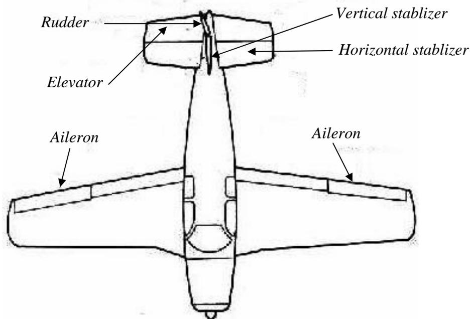
Fig (2.18) Control surfaces of an airplane.
