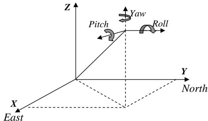
Fig (3.3) Flight parameters.
