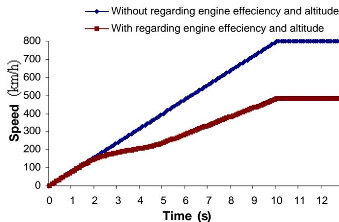
Fig (4.57) The effect of both high altitude and low engine efficiency on the behavior of simulated speed.
