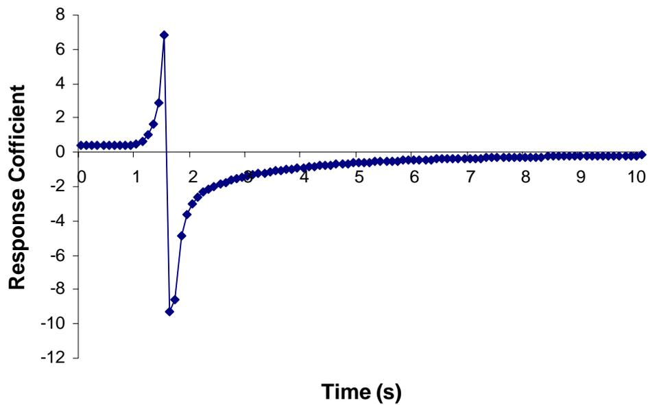
Fig (4.28) The response coefficient  $k_{22}$  computed by the simulated flight parameters.
