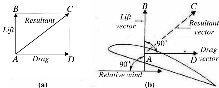
Fig (2.13): Relationship between relative wind, lift, and drag.
