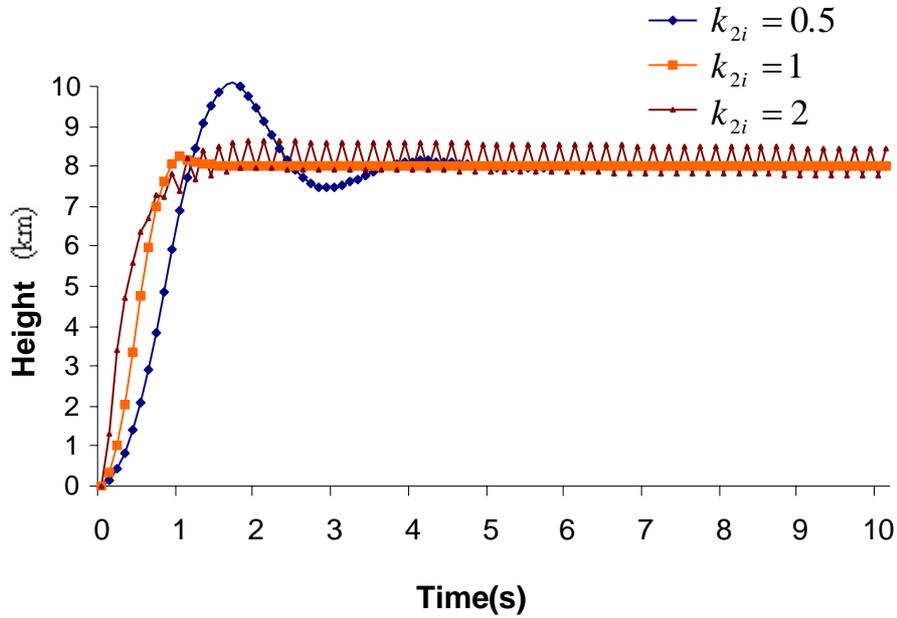
Fig (4.12) Simulated actual height behavior for different values of  $k_{2i}$ .
