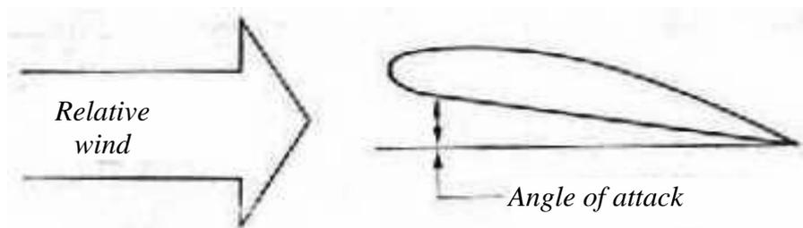
Fig (2.9) Angle of attack
