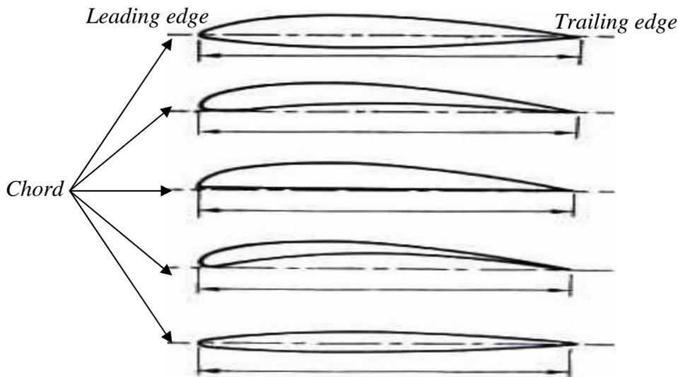
Fig (2.5) Airfoil profile of different shapes.
