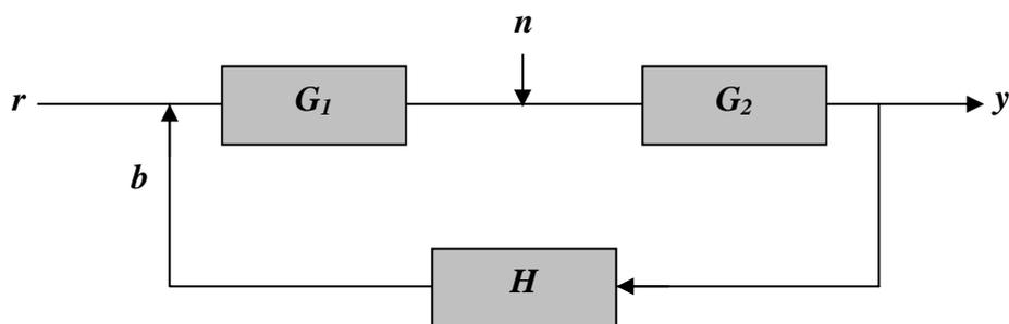
Fig (1.5) Feedback system with a noise signal.
