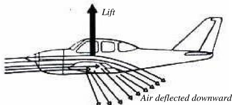
Fig (2.4) Wing deflecting the air downward.
