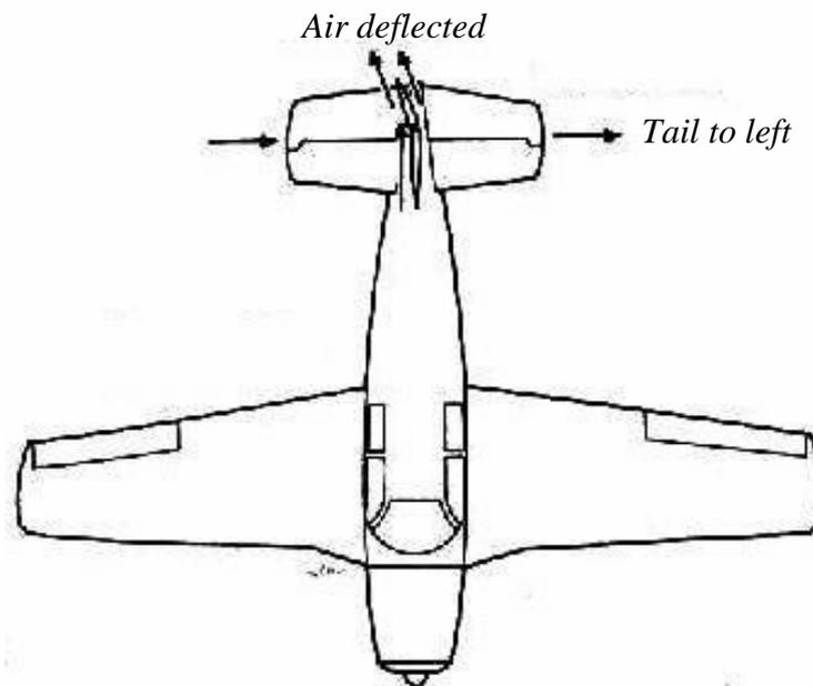
Fig (2.21) Action of the rudder.
