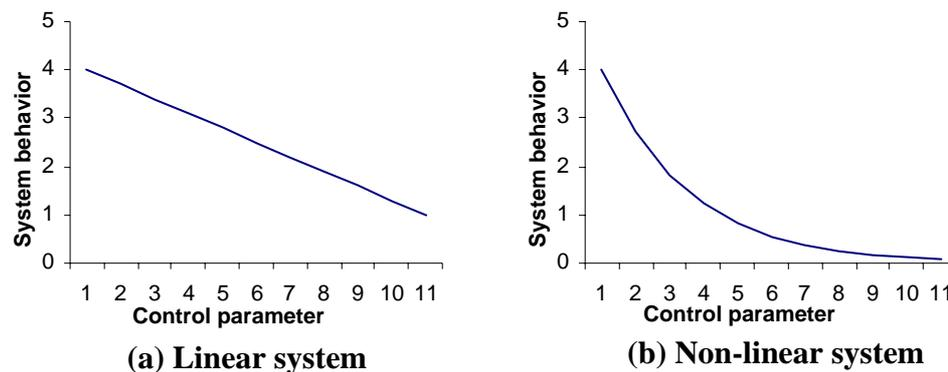
Fig (1.6) Linear and non-linear system behaviors.
