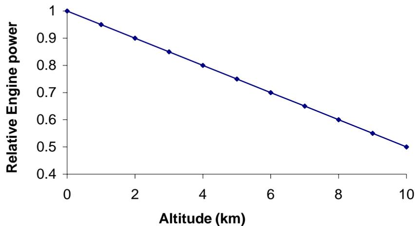
Fig (4.45) The relative engine power of the airplane versus altitude.
