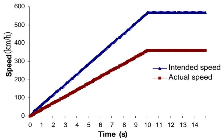
Fig (4.51) The behavior of simulated speed when the actual speed kept under the intended at high altitude.
