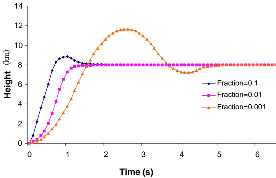
Fig (4.15) The effect of  $MaxChgF_2$  on the behavior of simulated height.
