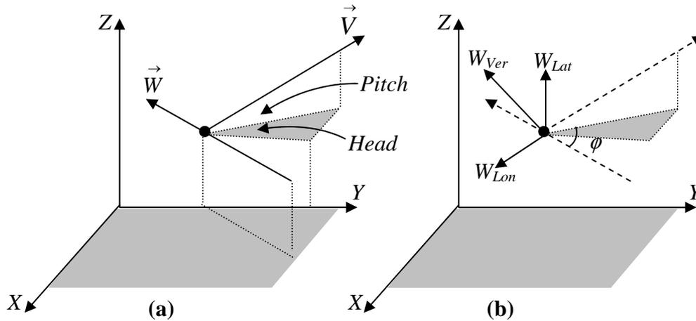
Fig (3.17) Components of wind speed with respect to the reference coordinates when the pitch and roll have non zero values.
