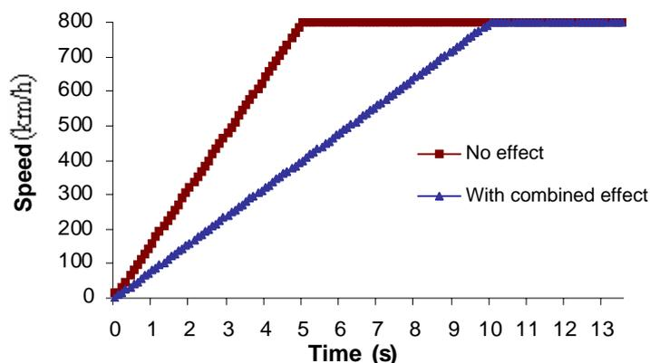
Fig (4.56) The effects of both low engine efficiency and opposite wind on the behavior of simulated speed.
