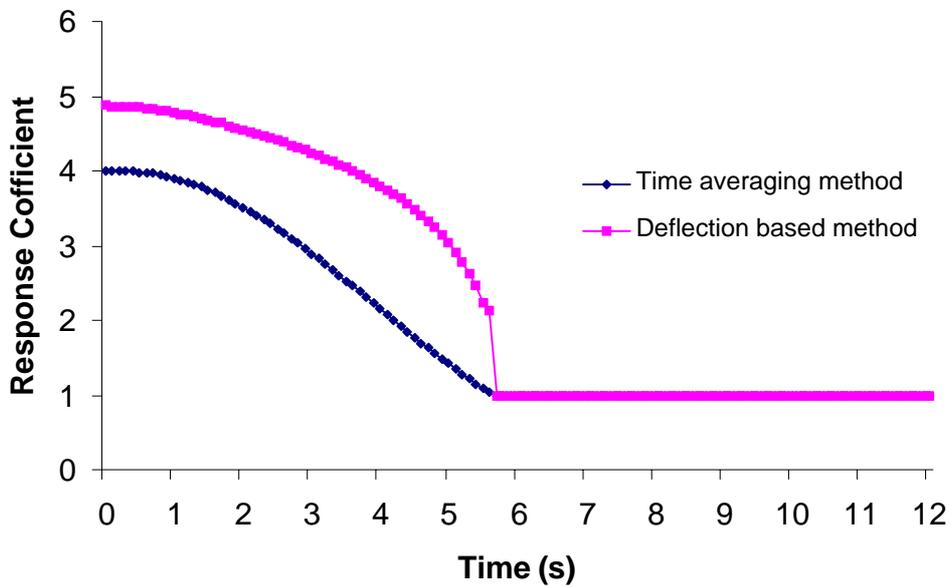
Fig (4.30) The response coefficient  $k_{22}$  computed by the simulated navigation parameters.
