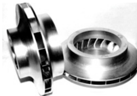
Figure 3.7 : EBW is suitable for fabricating high-strength stainless steel impellers for a centrifugal compressor [96].
