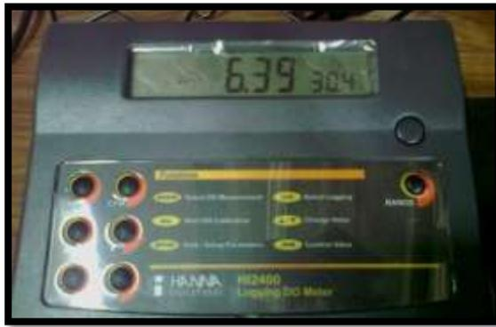
**Figure 3- 5** Dissolved oxygen meter
