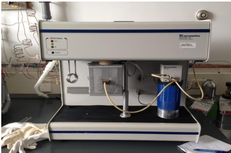
Image ( 2-5 ): Micromeritics AutoChem HP Chemisorption Analyzer (BET) (Karlsruhe Institute of Technology, Germany)
