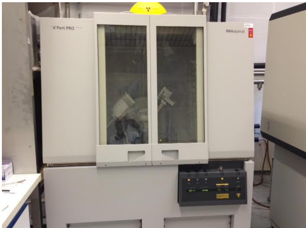
Image ( 2-3 ): Pananalytical Philips diffractometer (Karlsruhe Institute of Technology, Germany)
