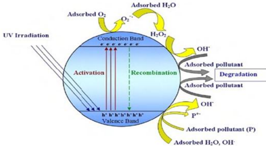
Figure (1-2): General mechanism of the photocatalysis on TiO 2 surface
