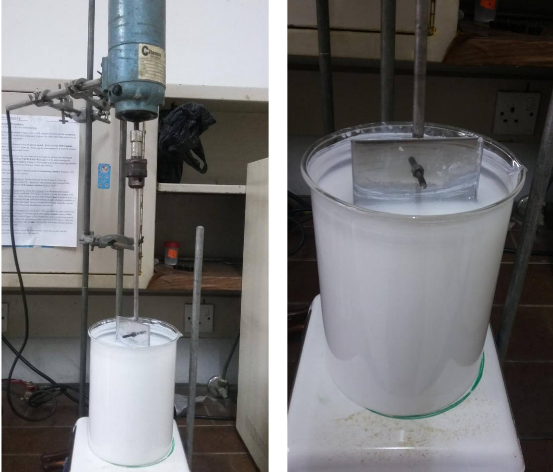
Figure ( 2-9 ): \text{TiO}_2 coating onto st. st. plate for prototype unit following rotation technique.
