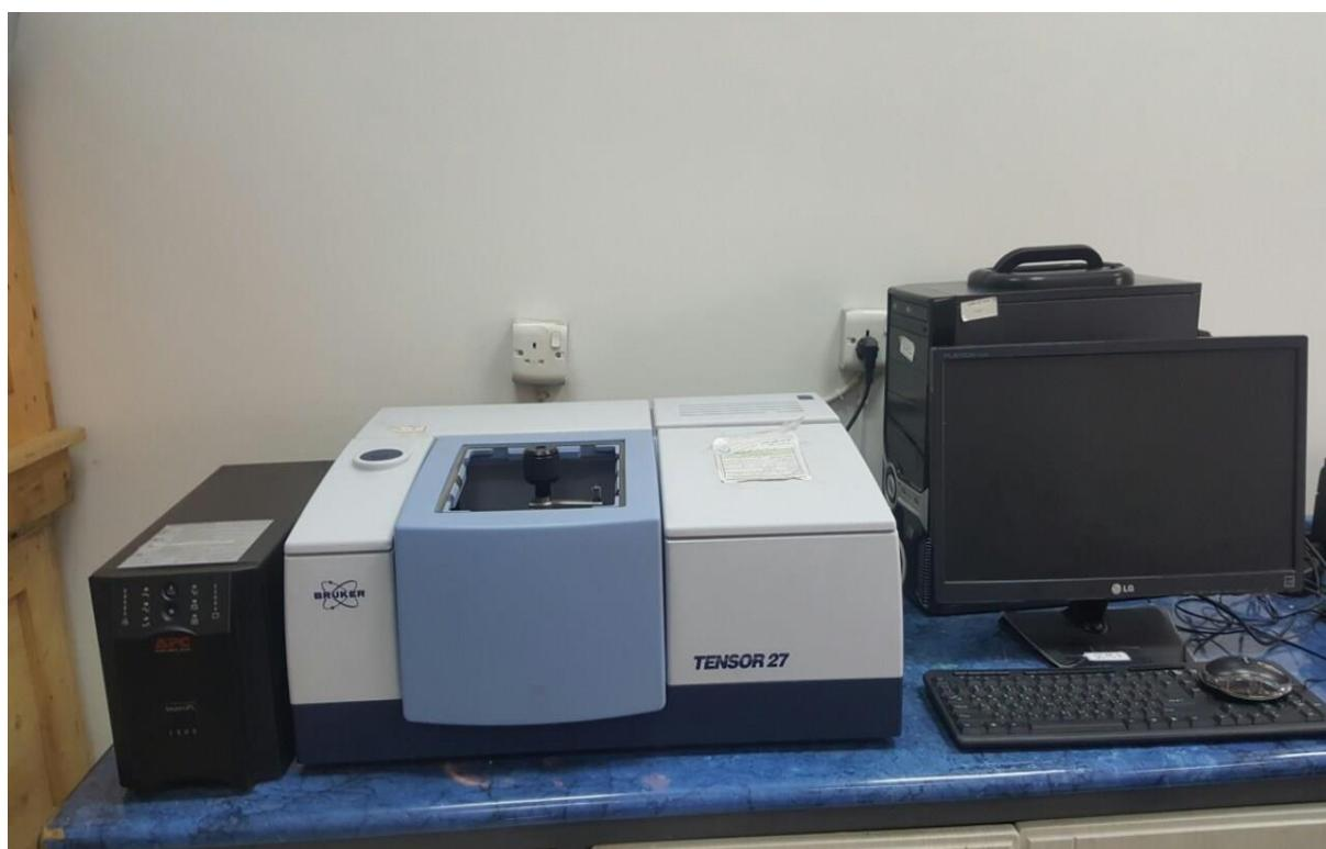
Figure (3- 3) FTIR spectroscopy model Tensor 27 from Bruker company, Germany.
