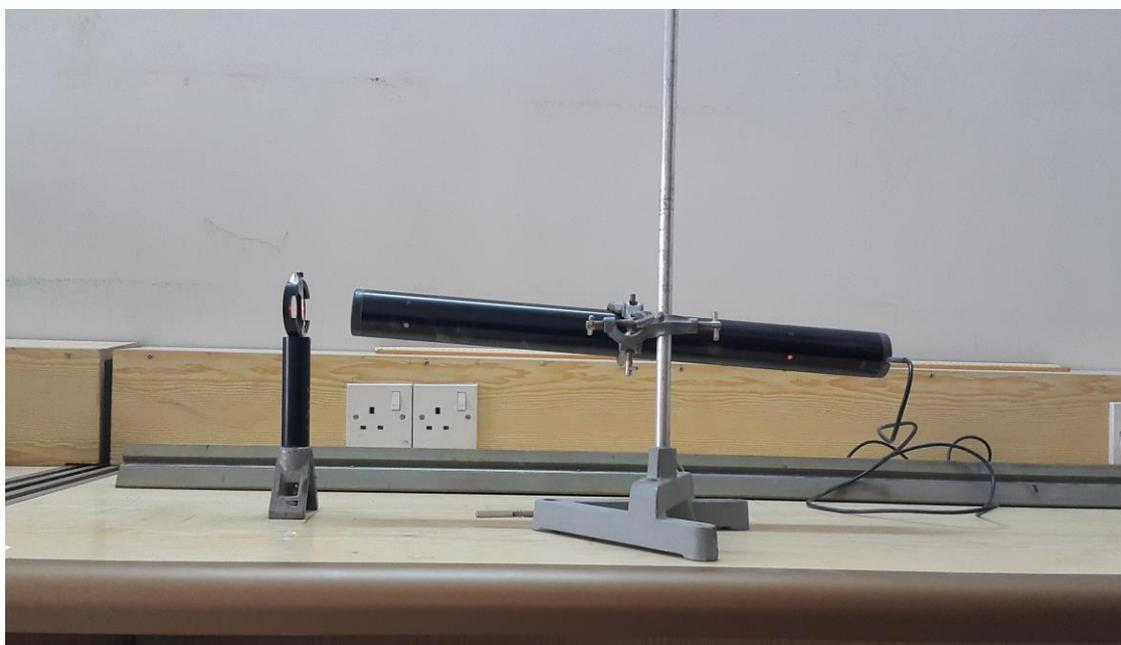
Figure (3-2) CR-39 irradiated with (He-Ne) laser beam.
