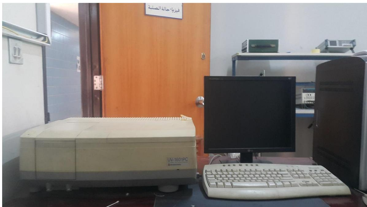
Figure (3-4) UV-Vis spectroscopy model SHIMADZU UV-1601PC UV-visible, Japan
