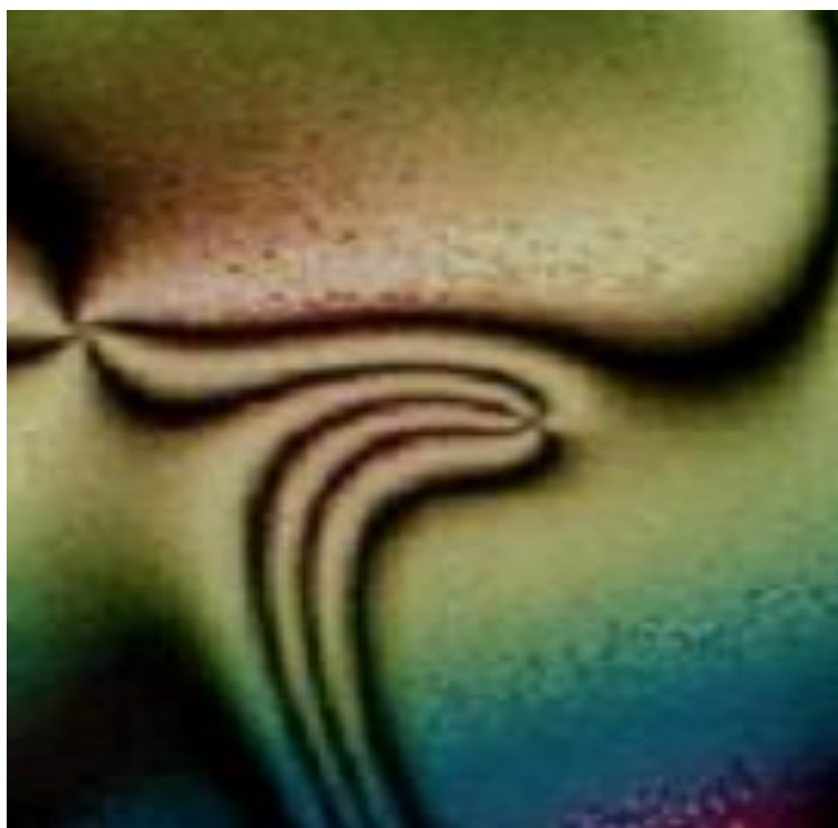
Figure (3.18): Nematic texture of N -{(n-propylxy-4'-bezoyloxy)-4'-benzylidene}-4-butyl aniline (4c).
