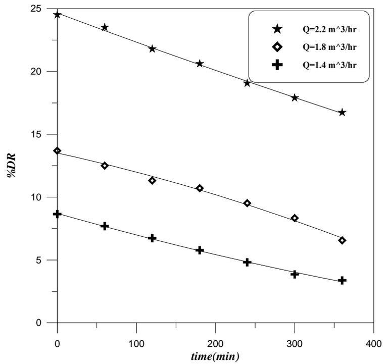
**Figure (4.16):** Effect of flow rate on polymer degradation for 25ppm PAAM
