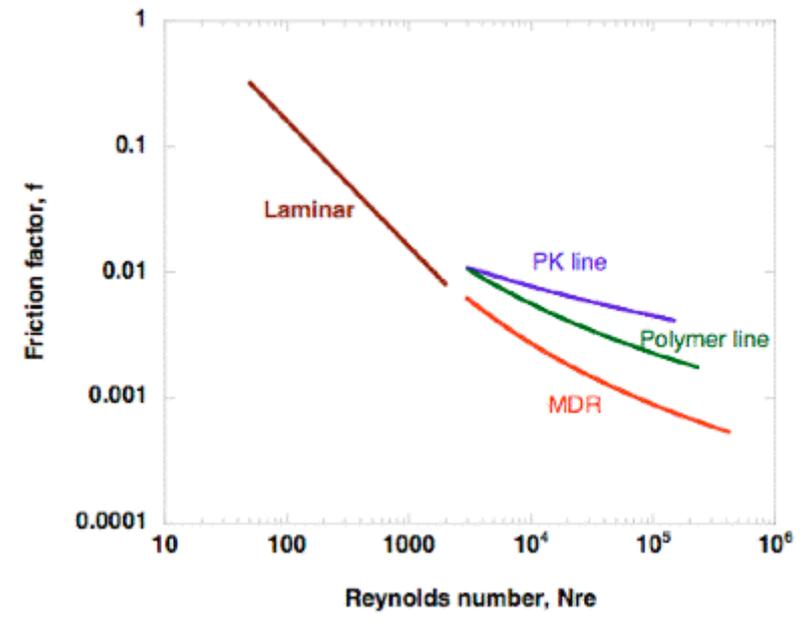
**Fig (2.1):**  $f$  vs  $Re$  plot depicting drag reduction. The polymer line is for some particular polymer, molar mass and concentration. Different concentrations, for example, will result in different polymer lines. The line labeled “PK” is for behavior of a Newtonian fluid<sup>(20)</sup>.
