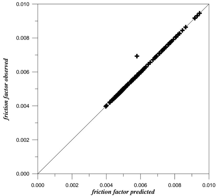
**Figure (4.37):** comparison of predicted and observed friction factor values polymer
