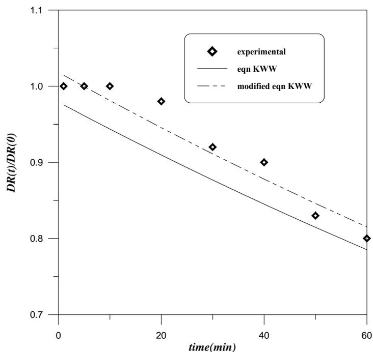
**Figure (4.38):**  $DR(t)/DR(0)$  as a function of time degradation, at 150 ppm PEO of a molecular weight= $4 \times 10^6$
