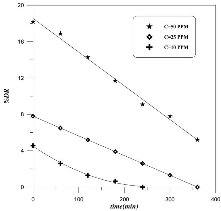
**Figure (4.31):** time-dependence of %DR at different PAAM additive,
