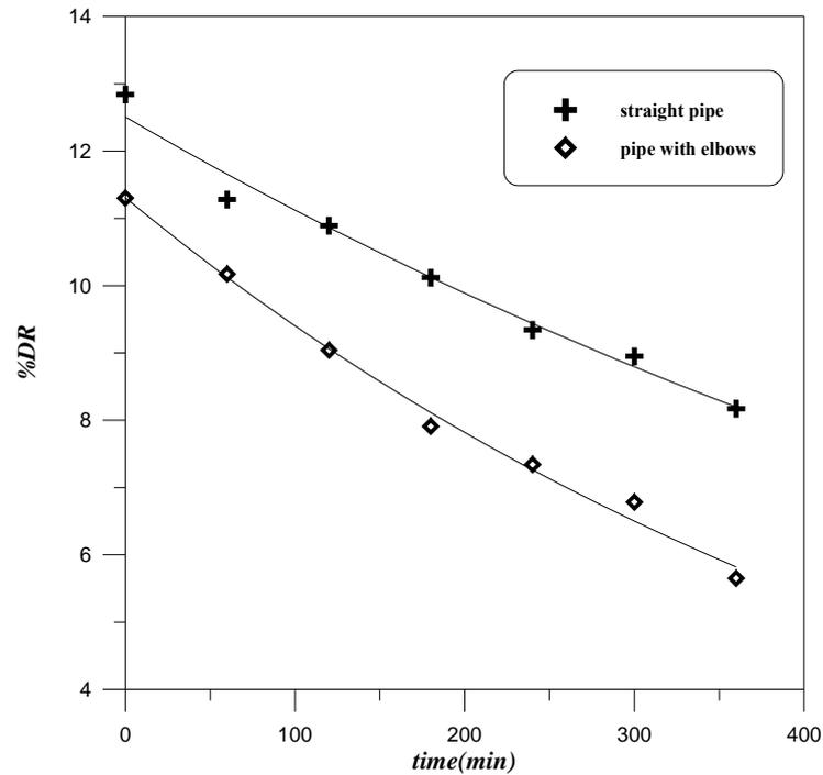
**Figure (4.30):** Effect of pipe type on degradation of XG at 150 ppm, 2.2 m<sup>3</sup>/hr
