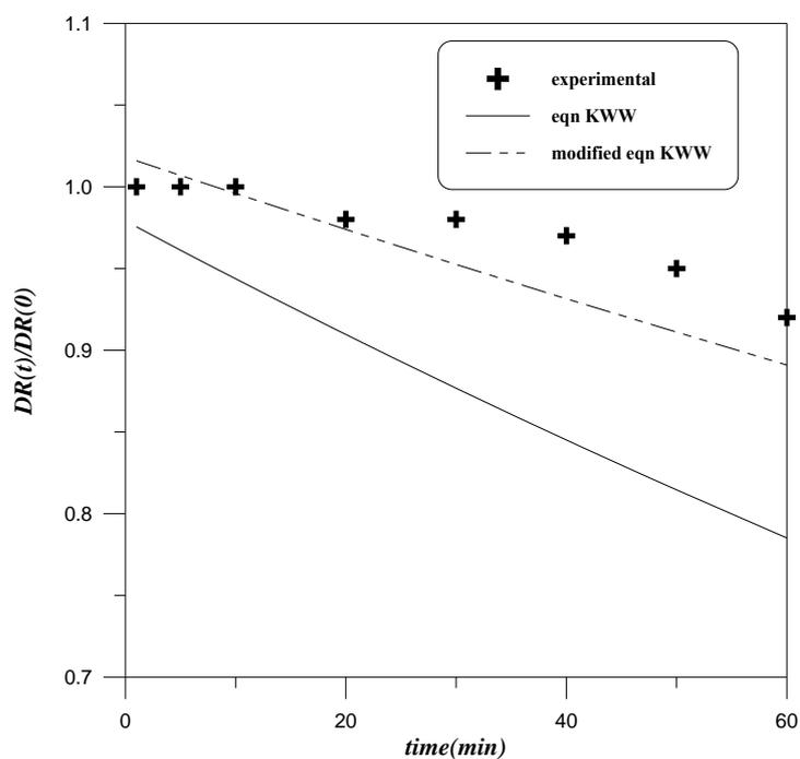
**Figure (4.39):**  $DR(t)/DR(0)$  as a function of time degradation, at 250 ppm PEO of a molecular weight= $4 \times 10^6$
