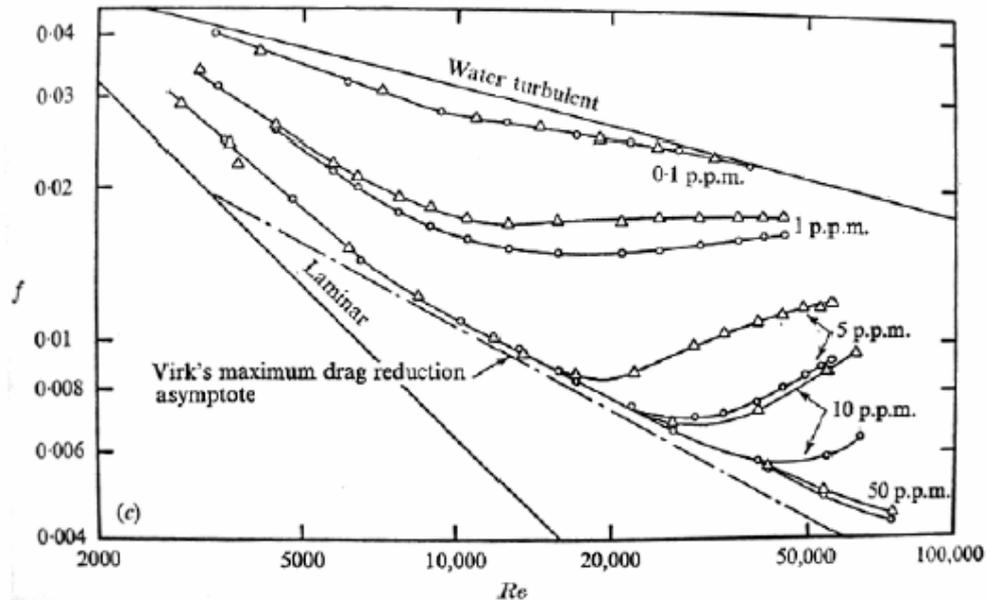
**Figure 2.4:** Friction factor plot for drag reduction and degradation of PEO MW=5\*10<sup>6</sup> g/mol, in a 6.29 mm ID pipe<sup>(38)</sup>.
