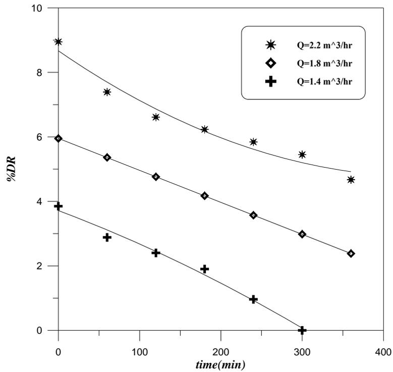
**Figure (4.10):** Effect of flow rate on polymer degradation for 100ppm XG
