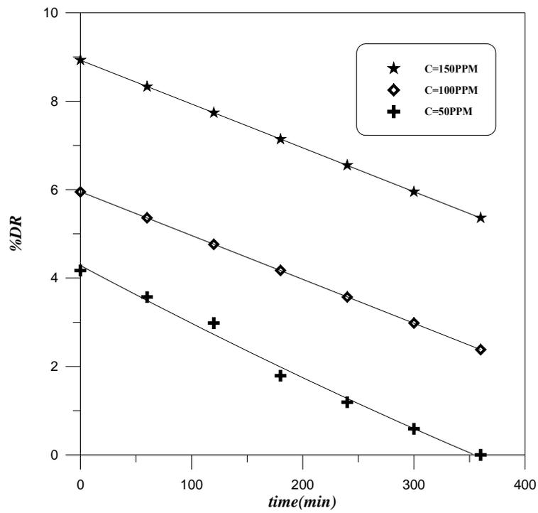
**Figure (4.13):** Effect of concentration of XG on polymer degradation at 1.8 m<sup>3</sup>/hr
