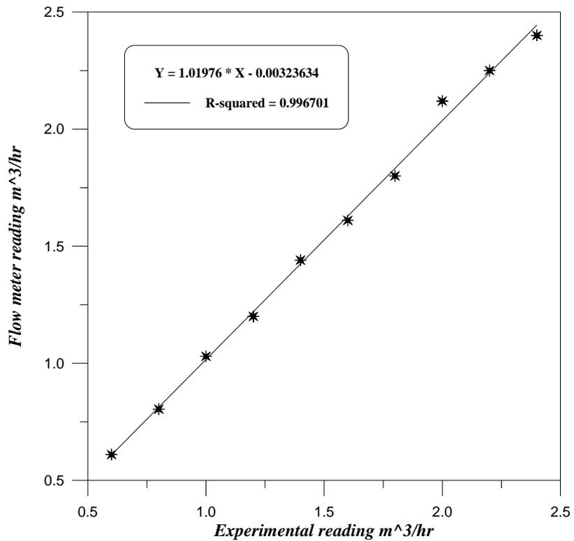
**Figure (3.2):** Calibration of flow meter
