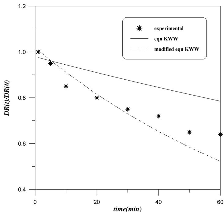
**Figure (4.40):**  $DR(t)/DR(0)$  as a function of time degradation, at 50 ppm PEO of a molecular weight  $=5 \cdot 10^6$
