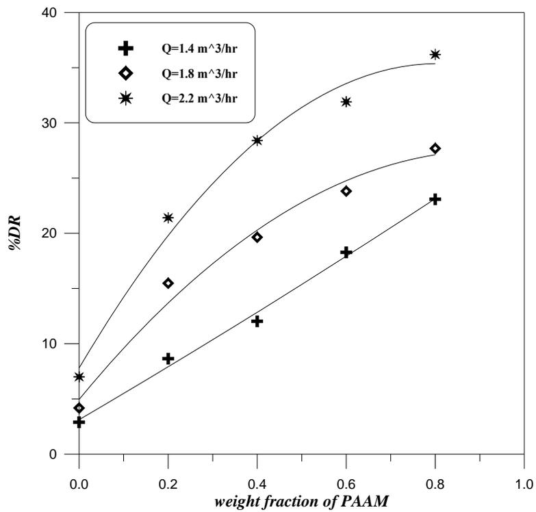
**Figure (4.6):** Effect of mixture composition at concentration=50 ppm on percent drag reduction
