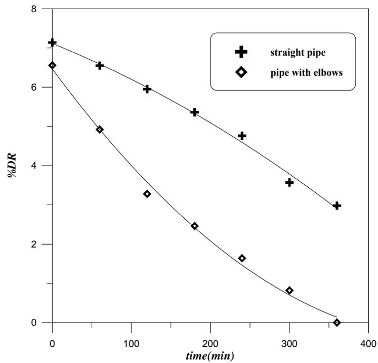
**Figure (4.34):** Effect of pipe type on degradation of PAAM at 10 ppm,
