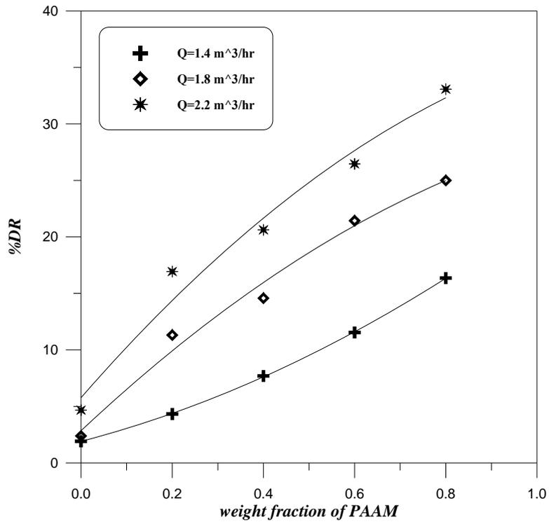
**Figure (4.5):** Effect of mixture composition at concentration=25 ppm on percent drag reduction
