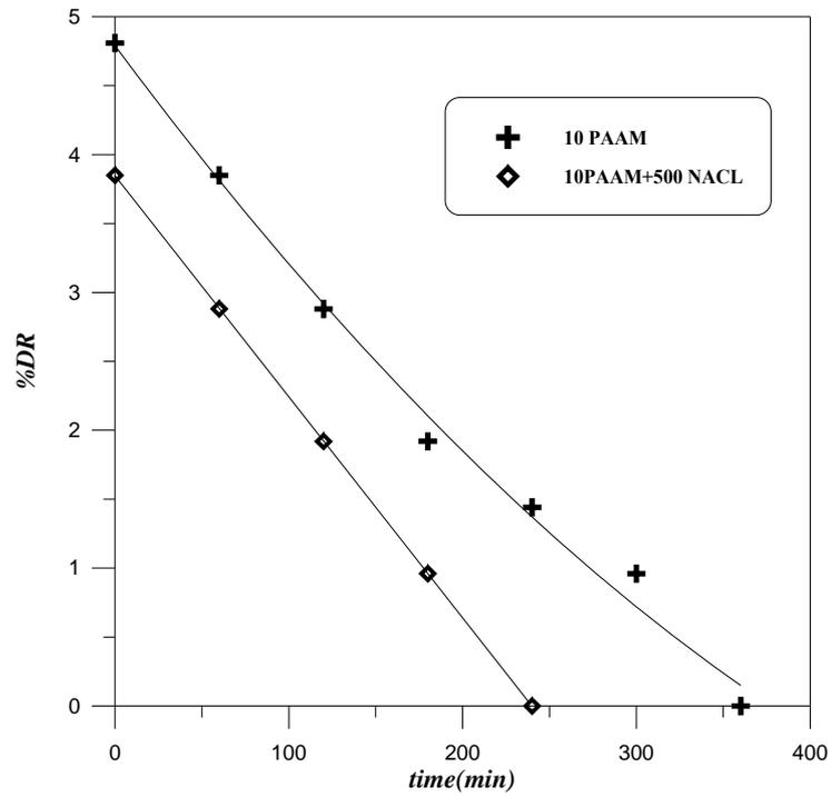
**Figure (4.21):** Effect of salt on polymer degradation for PAAM, at 1.4 m<sup>3</sup>/hr flow rate
