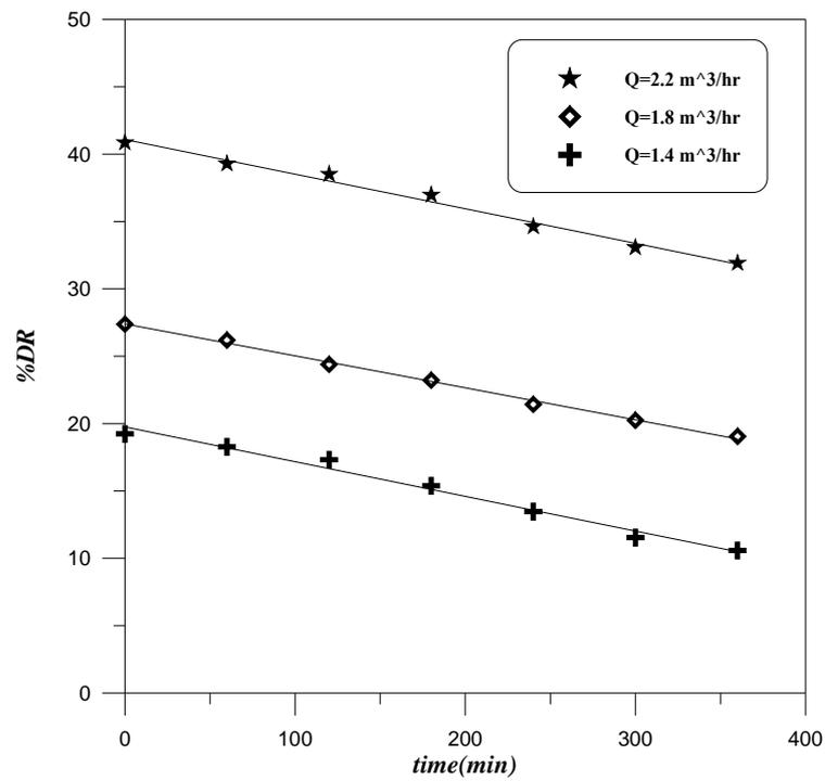
**Figure (4.17):** Effect of flow rate on polymer degradation for 50ppm PAAM
