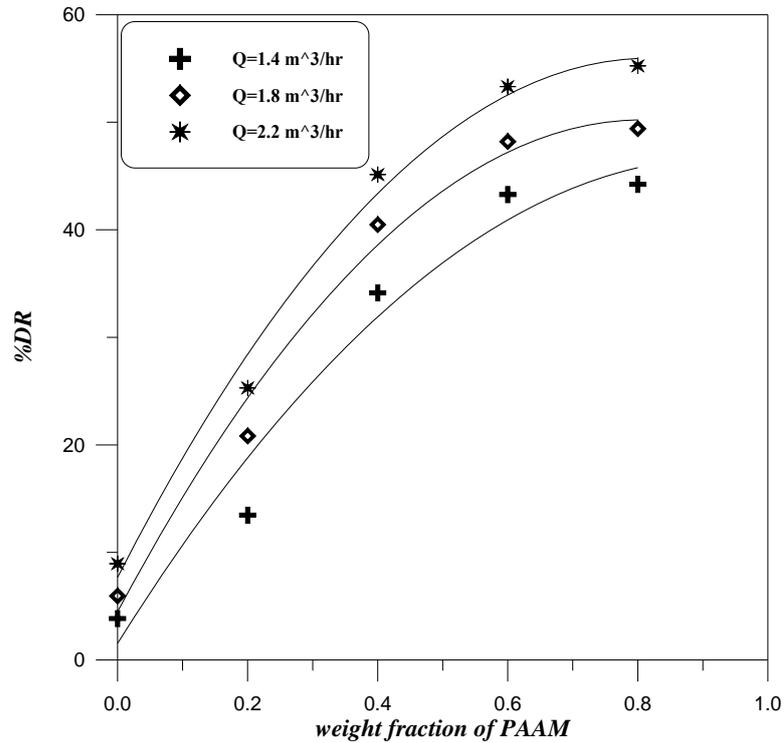
**Figure (4.7):** *Effect of mixture composition at concentration=100 ppm on percent drag reduction*
