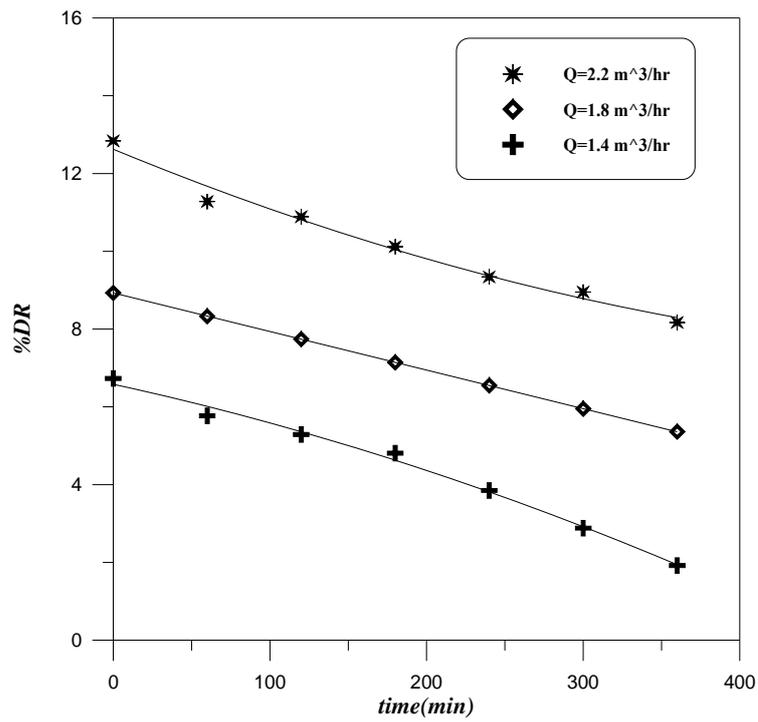
**Figure (4.11):** Effect of flow rate on polymer degradation for 150ppm XG
