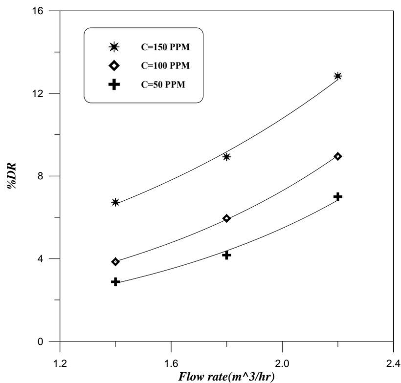
**Figure 4.2:** Effect of flow rate on percentage drag reduction for XG at different concentrations
