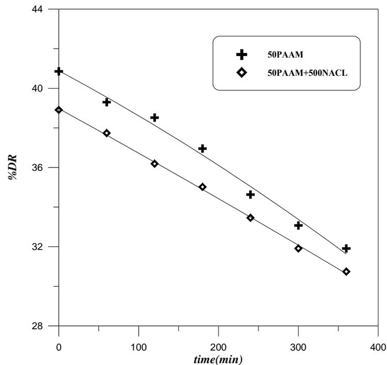
**Figure (4.23):** Effect of salt on polymer degradation for PAAM at 2.2 m<sup>3</sup>/hr flow rate
