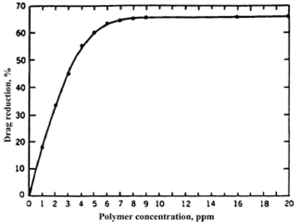
*Figure 2.3: Drag reduction of poly (ethylene oxide) in water, at a Reynolds number of 14000, in a small pipe<sup>(23)</sup>.*
