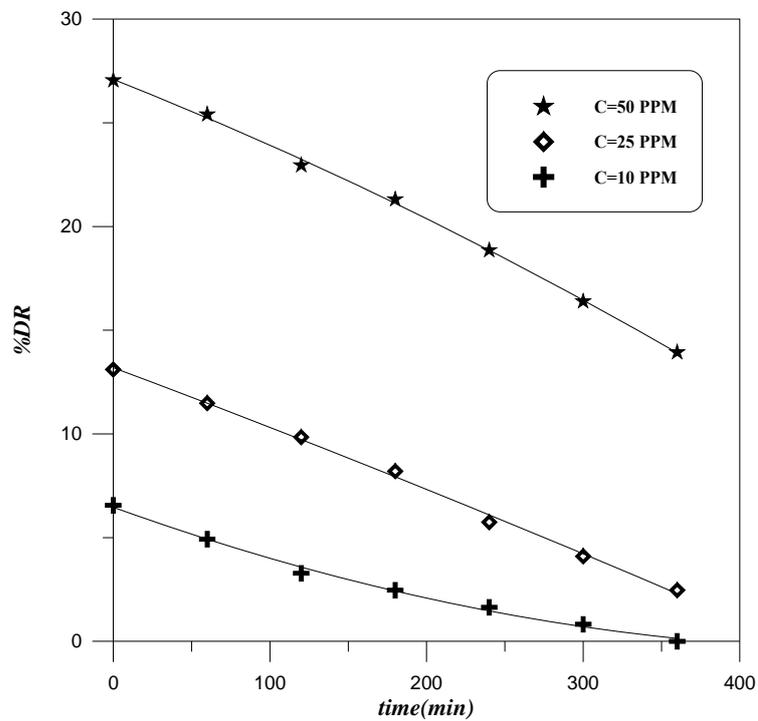
**Figure (4.32):** time-dependence of %DR at different PAAM additive,
