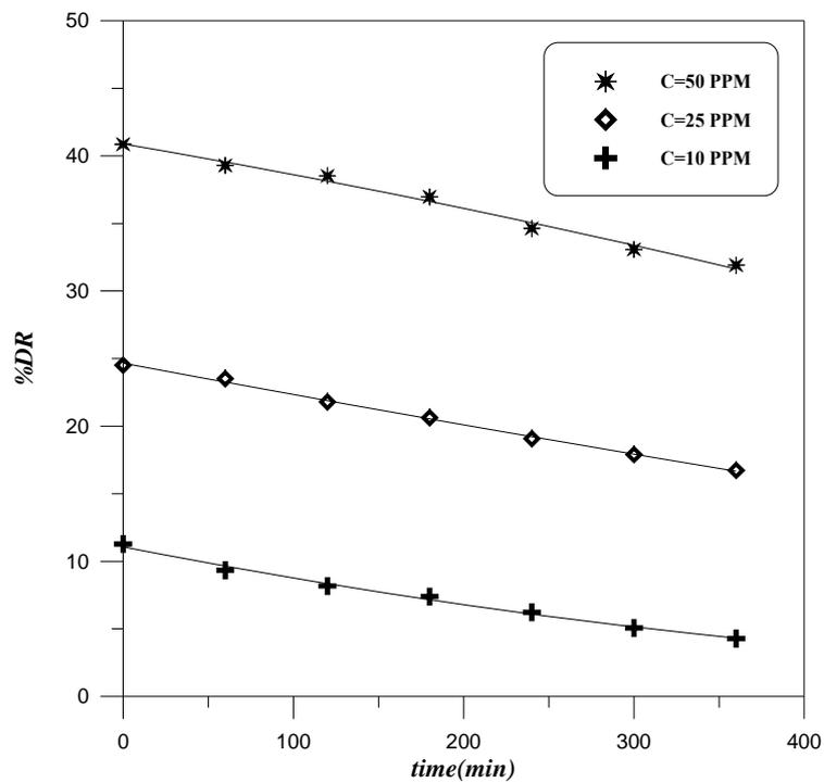
**Figure (4.20):** Effect of concentration of PAAM on polymer degradation at 2.2 m<sup>3</sup>/hr
