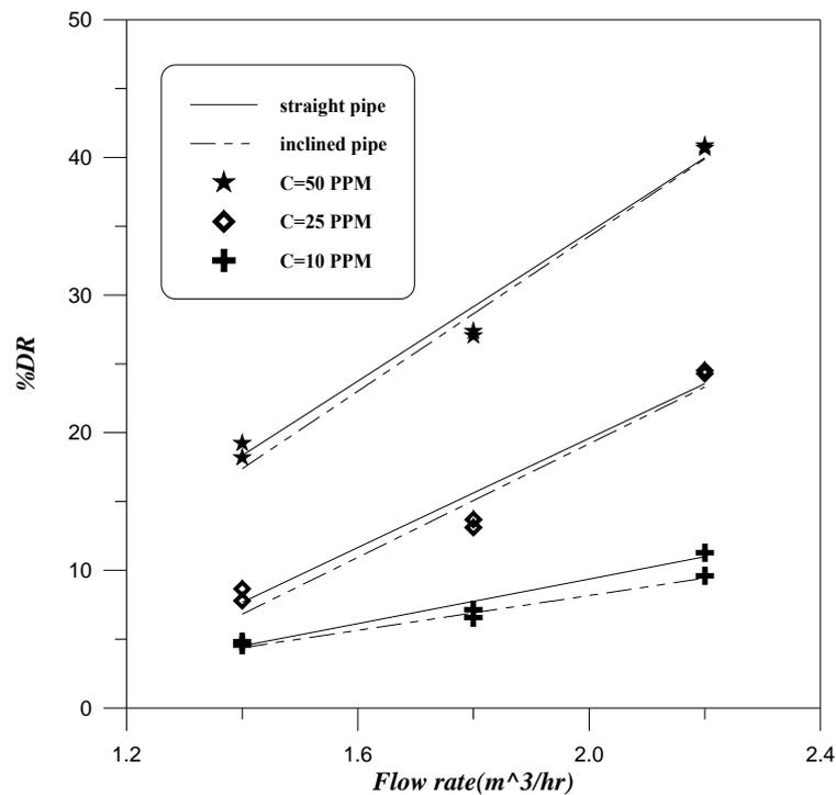
**Figure (4.25):** Effect of pipe configuration on drag-reduction efficiency of PAAM additive
