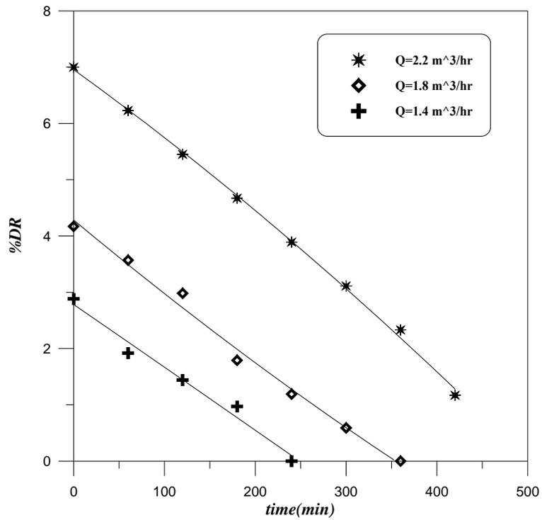
**Figure (4.9):** Effect of flow rate on polymer degradation for 50ppm XG
