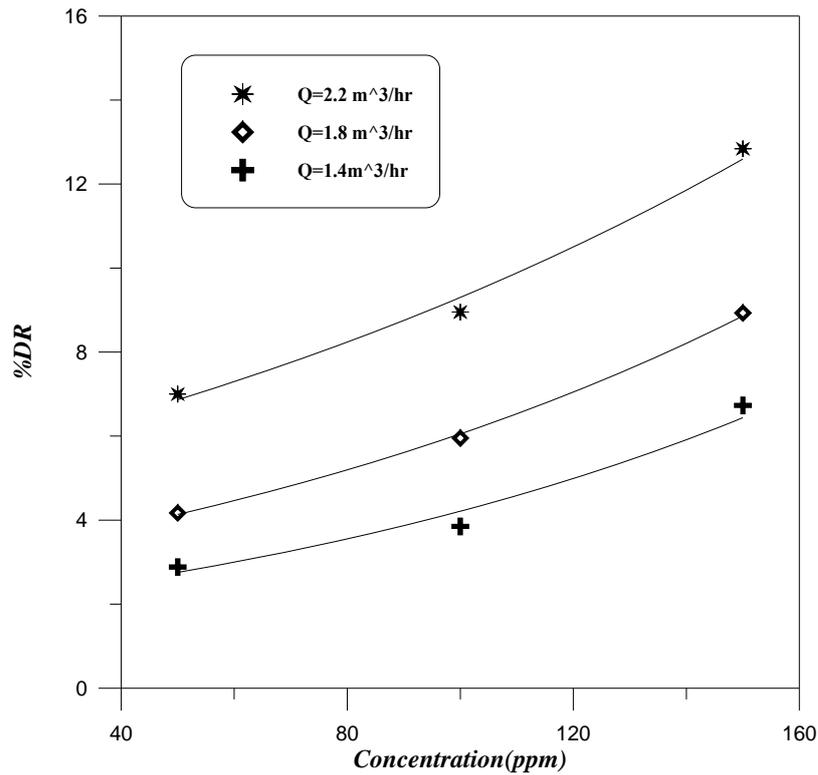
**Figure 4.1:** Effect of concentration on percentage drag reduction for XG at different flow rate
