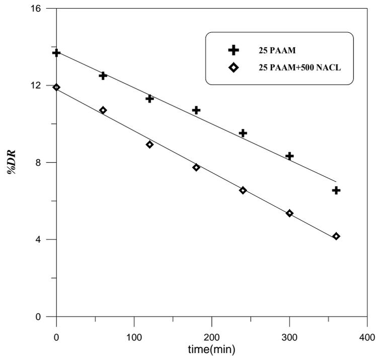
**Figure (4.22):** Effect of salt on polymer degradation for PAAM, at 1.8 m<sup>3</sup>/hr flow rate
