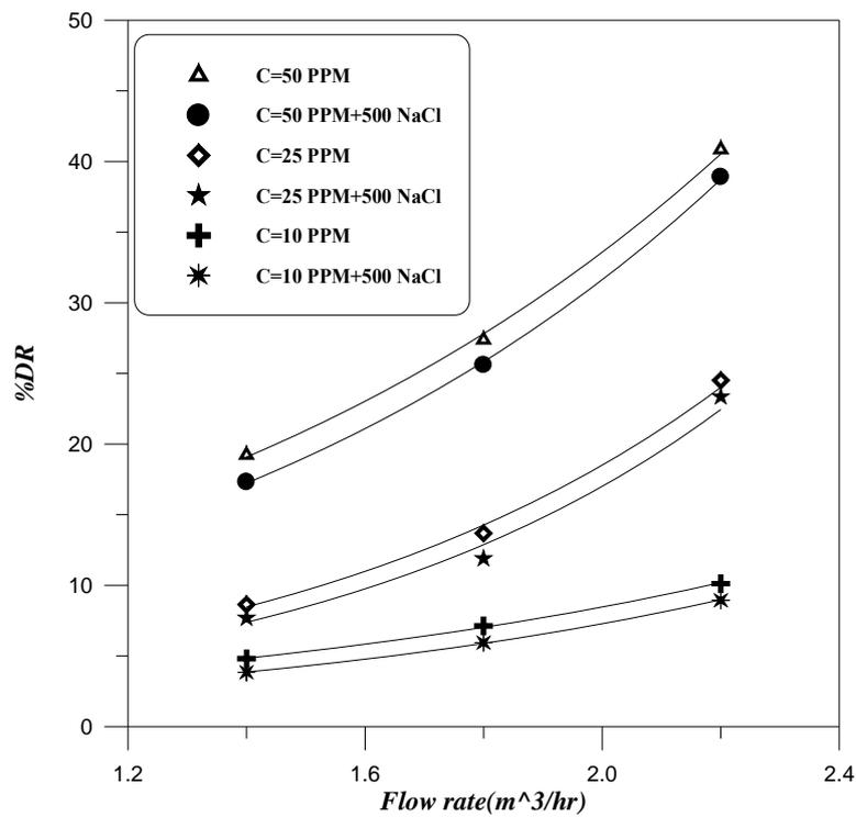
**Figure (4.8):** Effect of NaCl on percent drag reduction for PAAM
