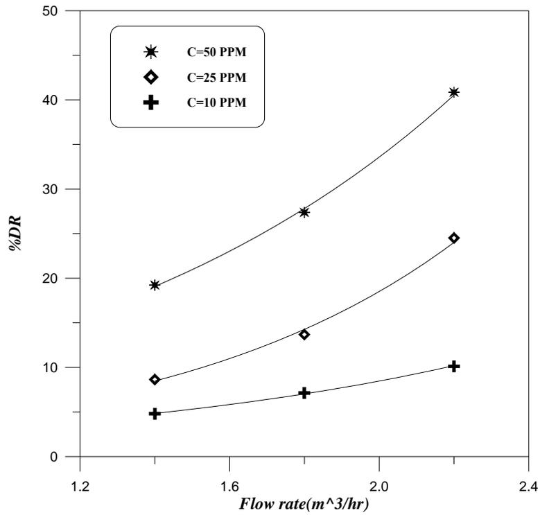
**Figure (4.3):** Effect of flow rate on percent drag reduction for PAAM
