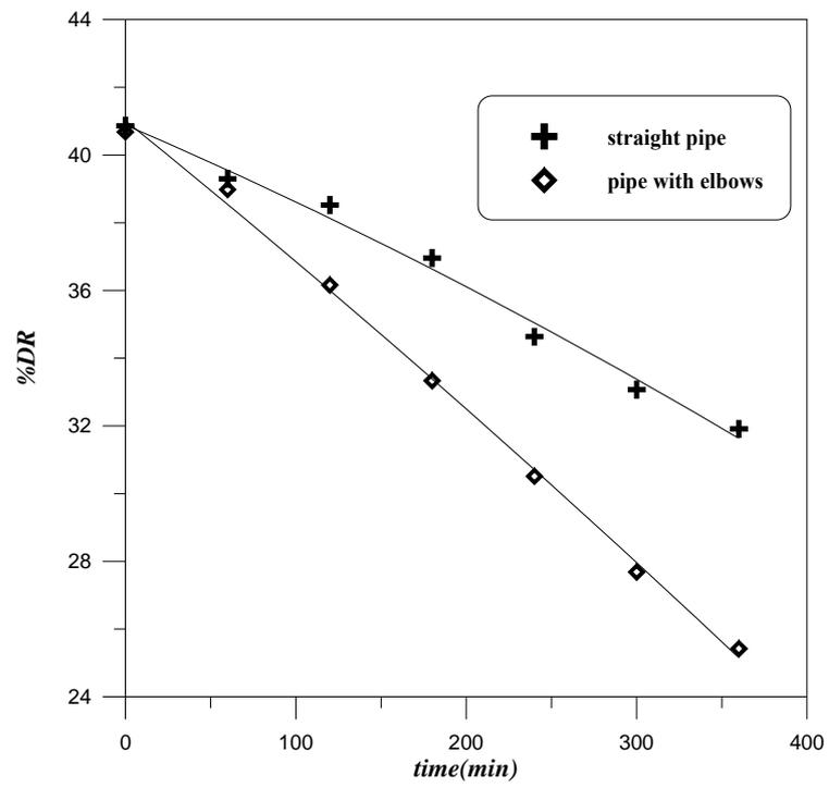
**Figure (4.35):** *Effect of pipe type on degradation of PAAM at 50 ppm, 2.2 m<sup>3</sup>/hr*
