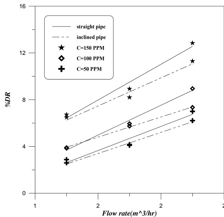
**Figure (4.24):** Effect of pipe configuration on drag-reduction efficiency of XG additive
