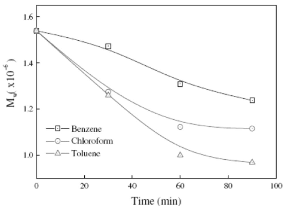
**Figure 2.7:** Solvent effect on the mechanical degradation of polystyrene <sup>(44)</sup>
