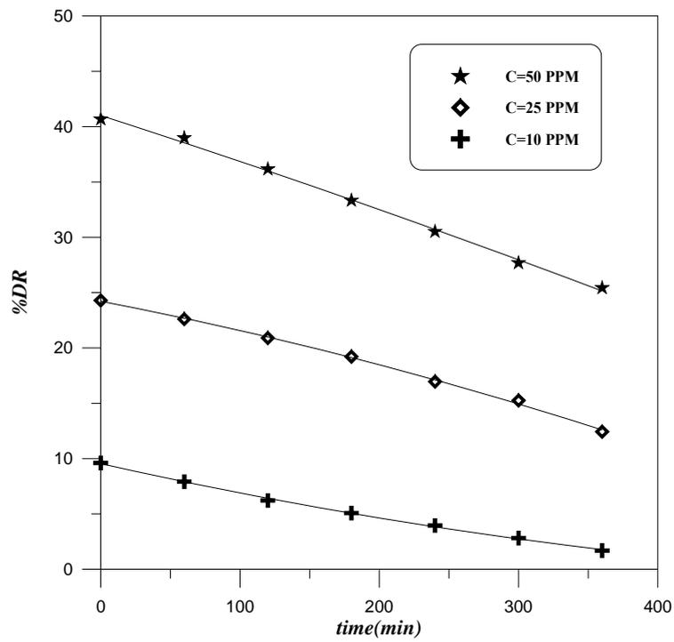
**Figure (4.33):** time-dependence of %DR at different PAAM additive,
