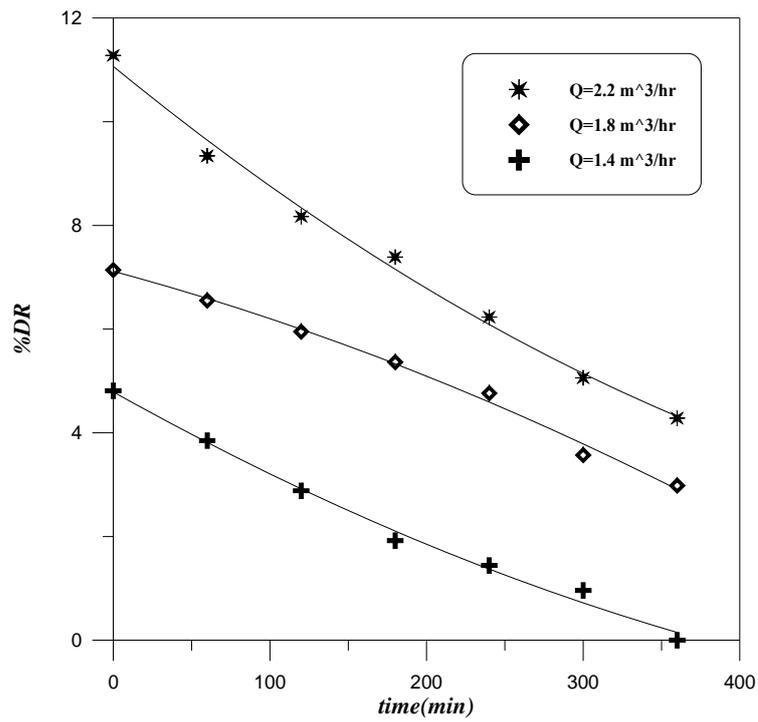
**Figure (4.15):** Effect of flow rate on polymer degradation for 10ppm PAAM
