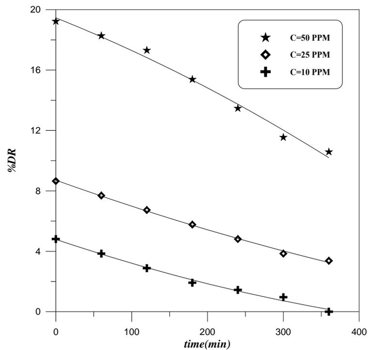
**Figure (4.18):** Effect of concentration of PAAM on polymer degradation at 1.4 m³/hr
