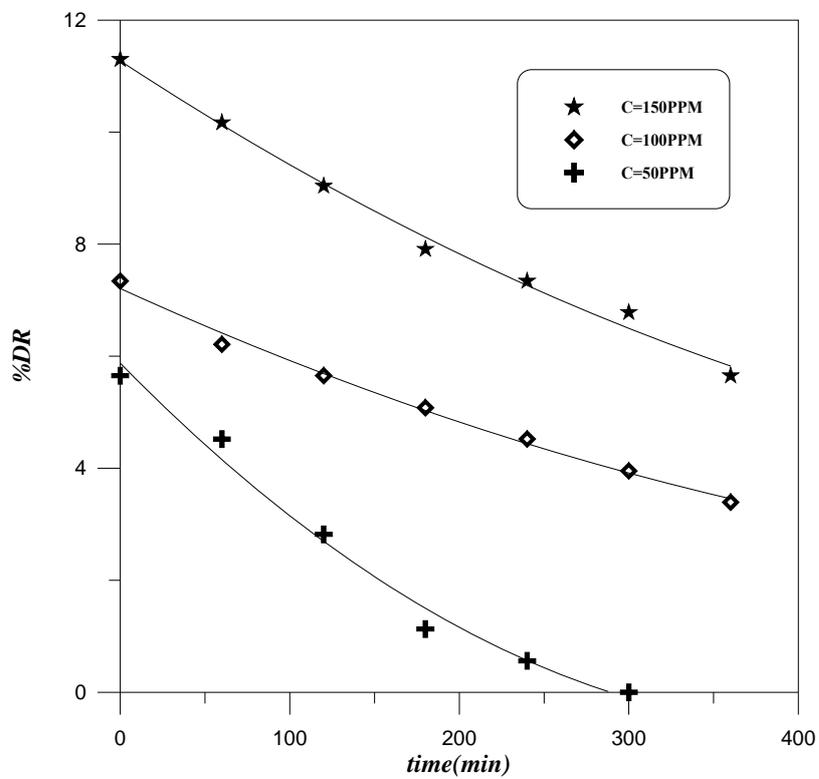
**Figure (4.28):** Effect of concentration on degradation of XG at  $Q=2.2\text{m}^3/\text{hr}$  in inclined pipe
