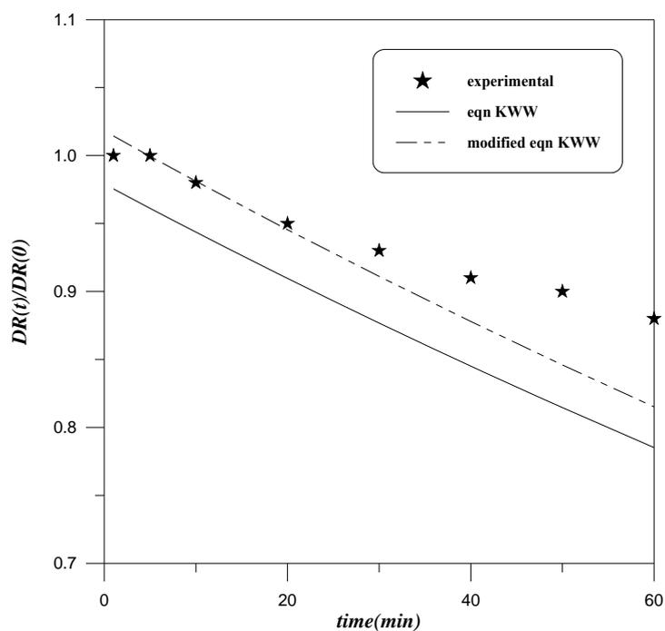
**Figure (4.41):**  $DR(t)/DR(0)$  as a function of time degradation, at 150 ppm PEO of a molecular weight  $=5 \cdot 10^6$
