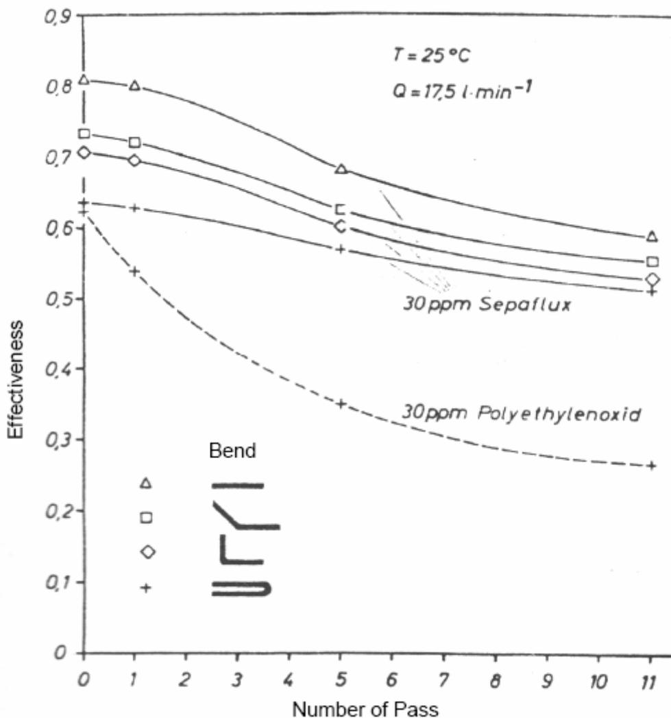
Figure 2.5: Effect of mechanical configuration on polymer effectiveness <sup>(42)</sup>.
