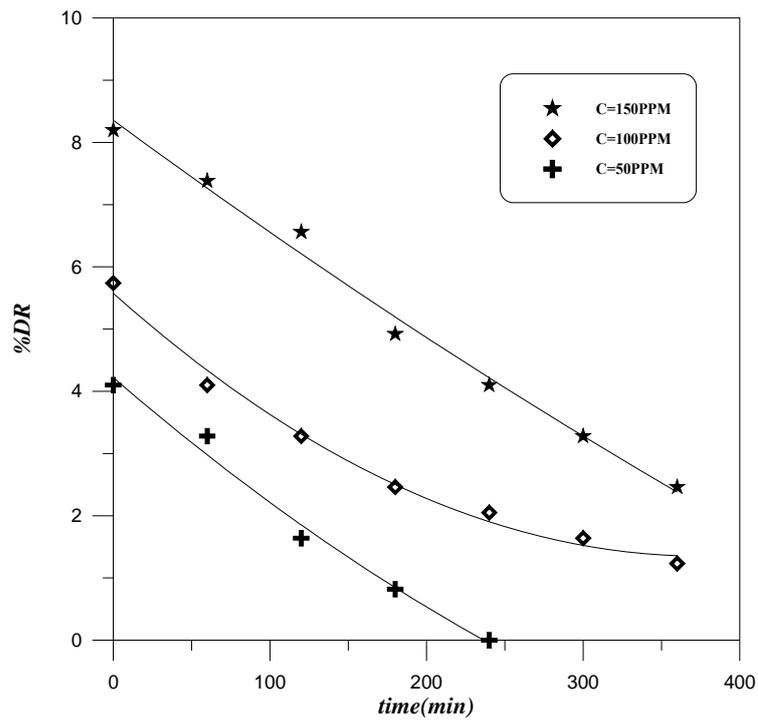
**Figure (4.27):** Effect of concentration on degradation of XG at  $Q=1.8\text{m}^3/\text{hr}$  in inclined pipe
