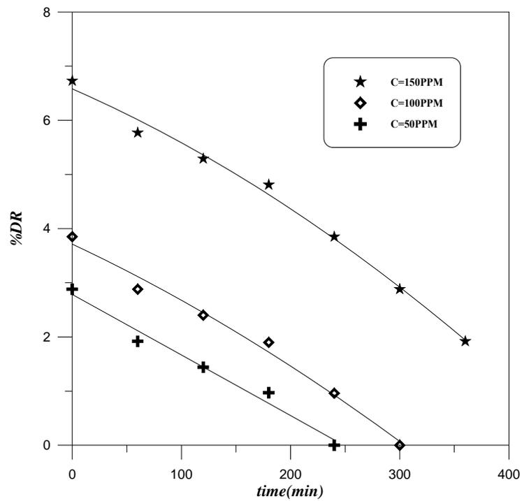
**Figure (4.12):** Effect of concentration of XG on polymer degradation at 1.4 m³/hr
