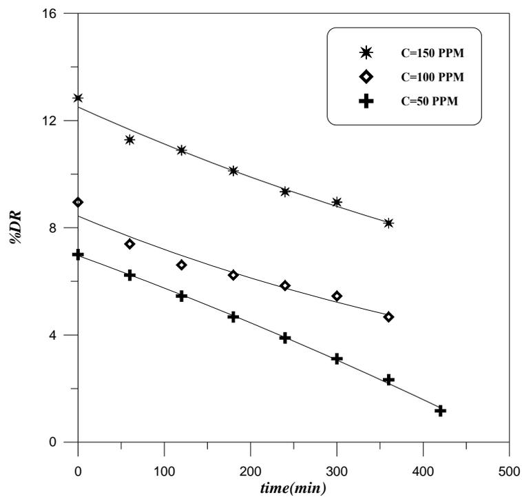
**Figure (4.14):** Effect of concentration of XG on polymer degradation at 2.2 m<sup>3</sup>/hr
