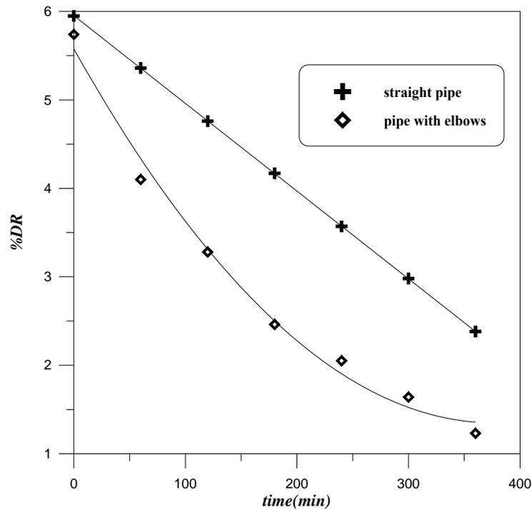
**Figure (4.29):** Effect of pipe type on degradation of XG at 100 ppm, 1.8 m<sup>3</sup>/hr
