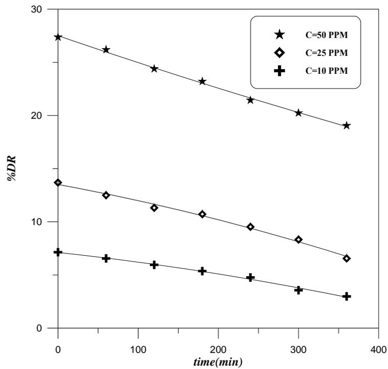
**Figure (4.19):** Effect of concentration of PAAM on polymer degradation at 1.8 m<sup>3</sup>/hr
