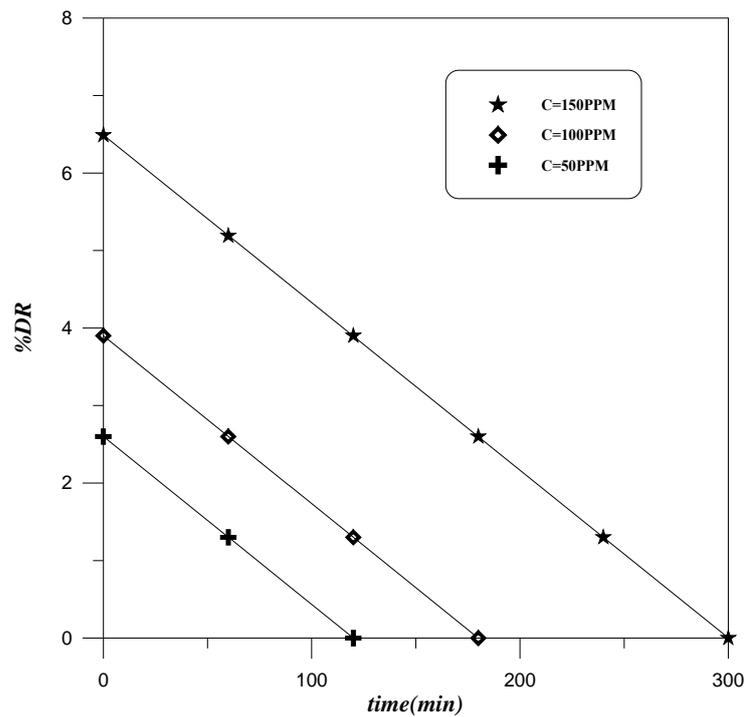
**Figure (4.26):** Effect of concentration on degradation of XG at  $Q=1.4\text{m}^3/\text{hr}$  in inclined pipe
