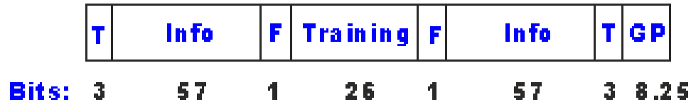
Figure 3-10 GSM Normal Burst
