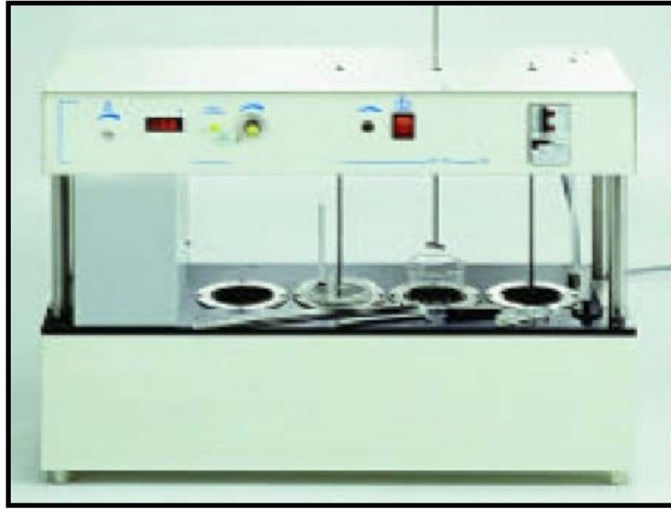
Fig. (3.2) Rust Preventing Tester of Inhibited Mineral Oil in the Presence of Water.
