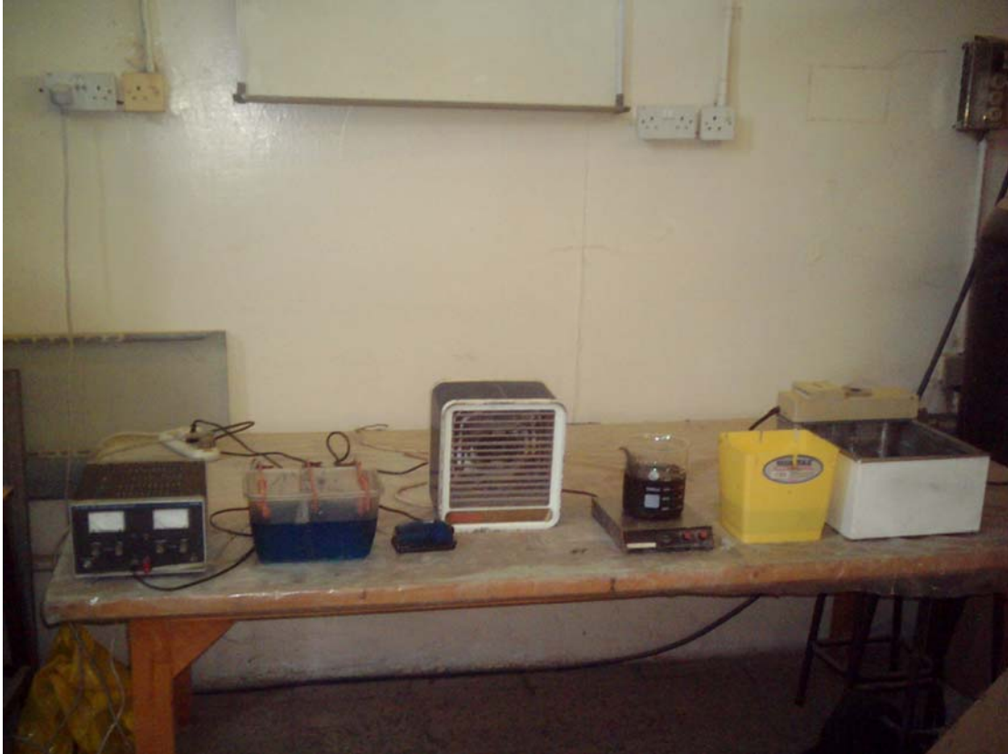
Figure 3-2 Plating of Plastic System
