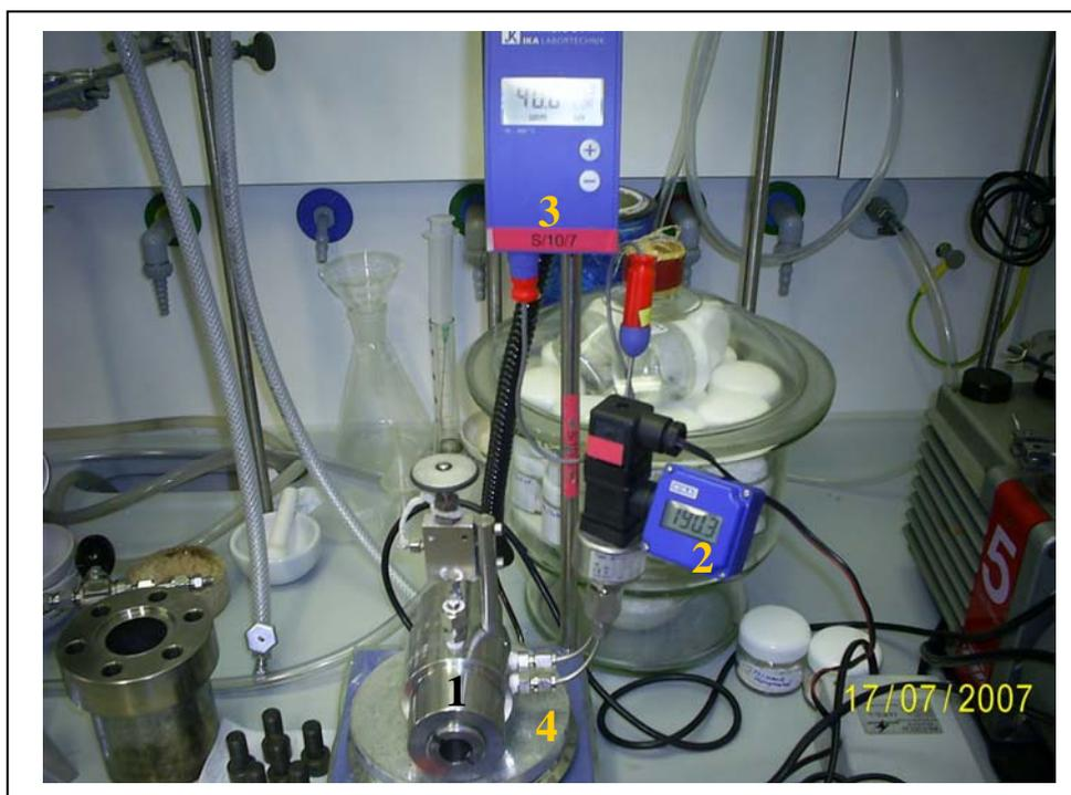
**Figure 4-3:** Photo picture for metal loading setup, 1- Body of autoclave, 2-digital manometer, 3- thermocouple, 4- magnetic stirrer
