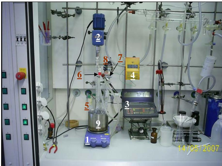
*Figure 4-1b:* The apparatus of ion exchange using Batch Wise
