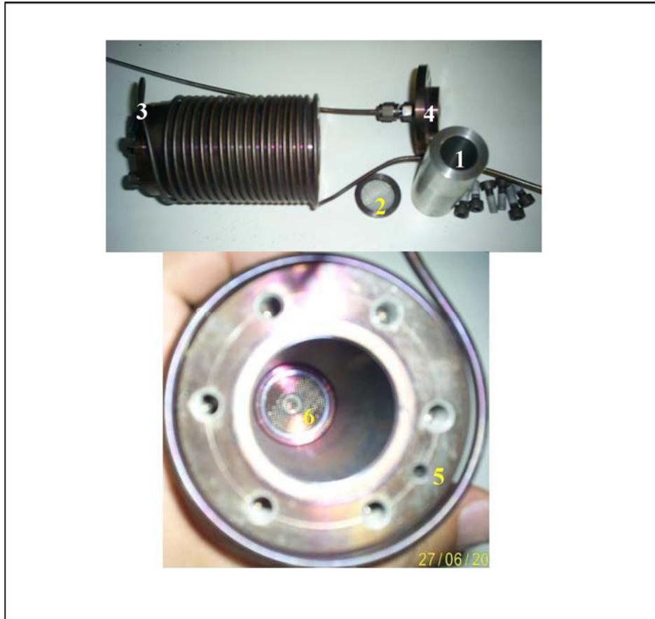
**Figure 4-11:** Picture for the reactor that used for reduction and reaction, 1- Hollow beam represents inner diameter of reactor, 2- upper sieve, 3- feed from down, 4- upper cover for reactor, 5- hole for thermocouple to the center, 6- down sieve.
