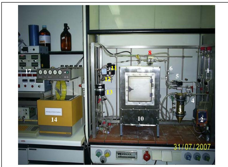
**Figure 4-10:** Photo Picture for the Flow Diagram of Catalytic Study Rig,
