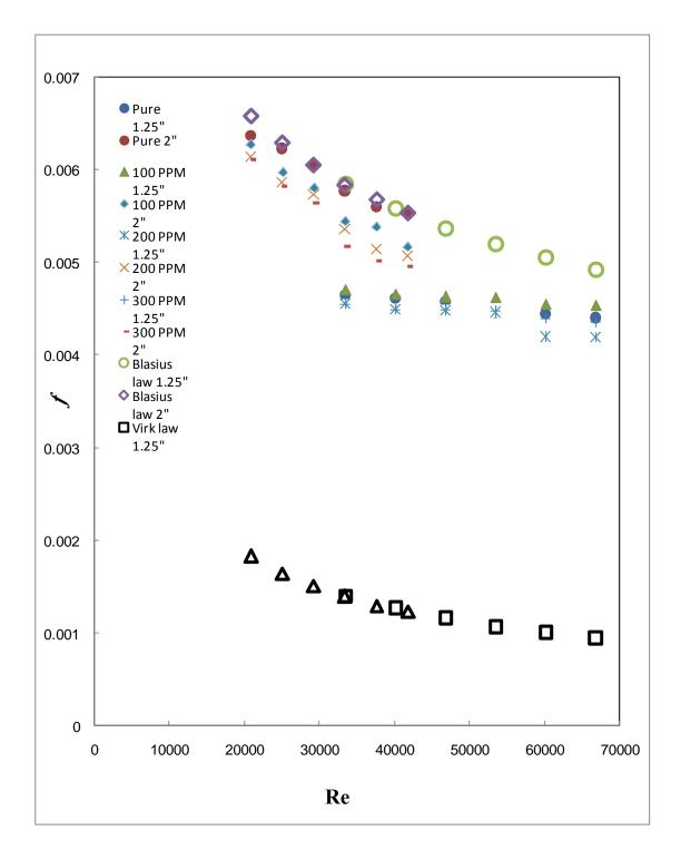
Fig. 4.36 Friction factor as function of Reynolds number for SS.
