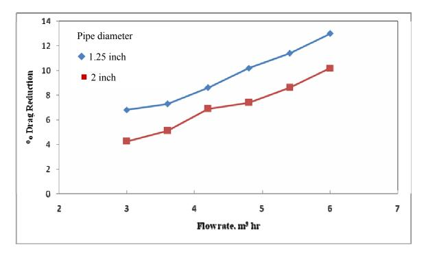
Fig. 4.3 Effect of flow rate on percentage drag reduction for CMC in a 200 ppm.
