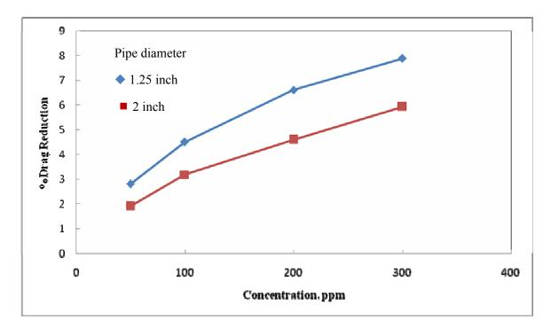
Fig. 4.10 Effect of concentration on percentage drag reduction for SLS at 6m<sup>3</sup>/hr.
