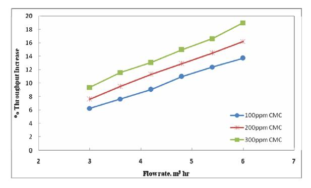
**Fig. 4.34** Effect of adding CMC on percentage throughput increase for water – clay suspension with solid concentration of 5000ppm through 2inch I.D pipe.
