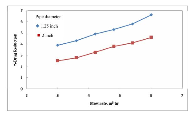
Fig. 4.14 Effect of flow rate on percentage drag reduction for SLS in a 200 ppm.
