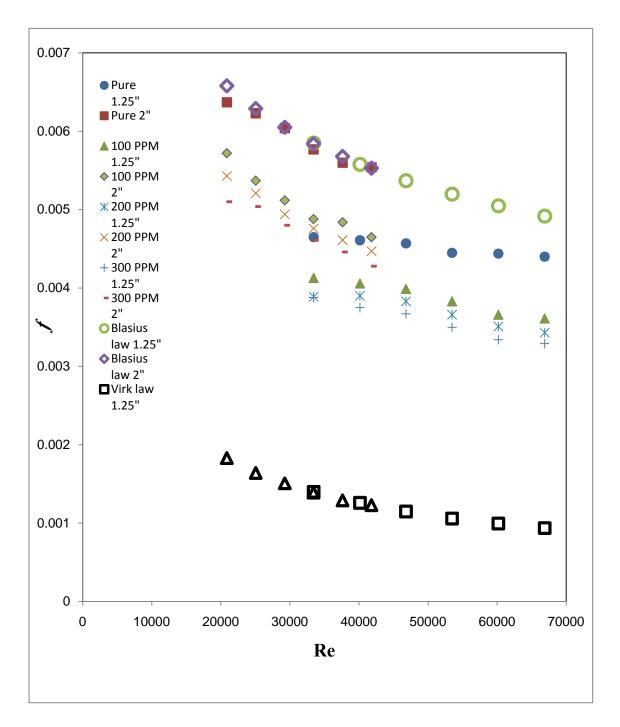
**Fig. 4.38** Friction factor as function of Reynolds number for adding CMC in water – clay suspension.
