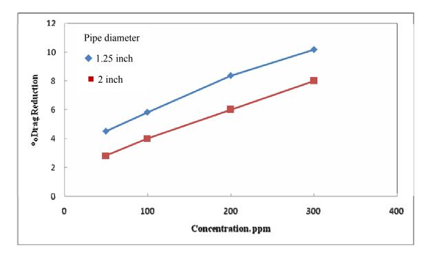
Fig. 4.8 Effect of concentration on percentage drag reduction for SS at 6m<sup>3</sup>/hr.
