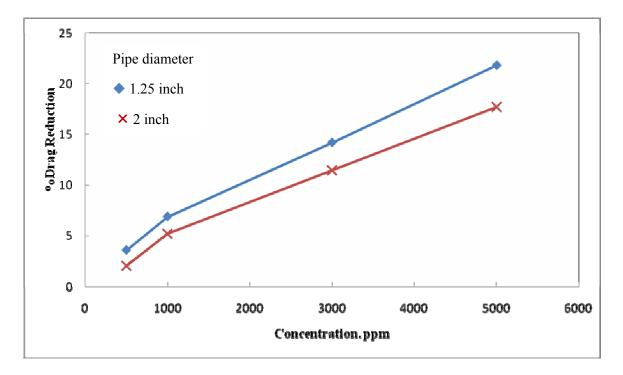
**Fig. 4.24** Effect of concentration on percentage drag reduction for transported water with clay as suspended solid at 6m<sup>3</sup>/hr.
