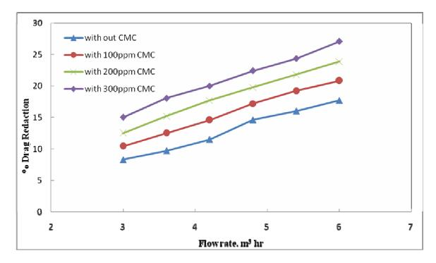
**Fig. 4.31** Effect of adding CMC on percentage drag reduction for water – clay suspension with solid concentration of 5000ppm through 2inch I.D pipe
