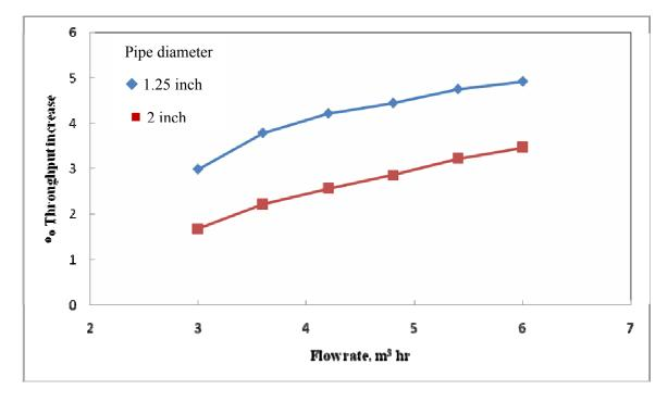
Fig. 4.15 Effect of flow rate on percentage throughput increase for SS in a 200 ppm.
