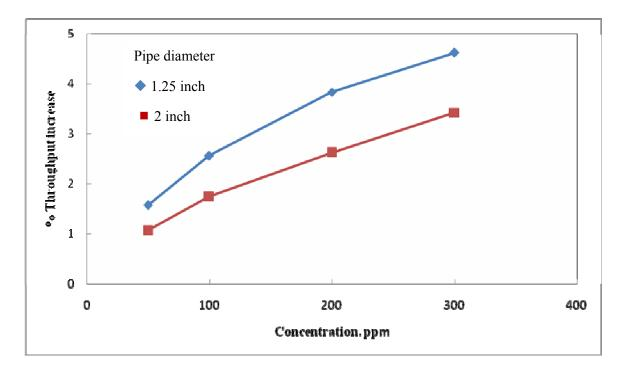
Fig. 4.12 Effect of concentration on percentage throughput increase for SLS at  $6m^3/hr$ .
