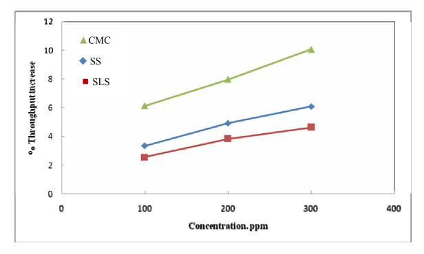
**Fig. 4.19** Effect of concentration on percentage throughput increase for SS, SLS surfactants and CMC polymer at 6.0 m<sup>3</sup>/hr through 1.25 inch I.D pipe.
