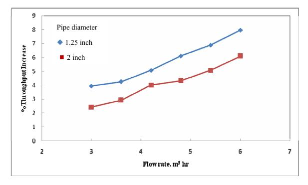
**Fig. 4.6** Effect of flow rate on percentage throughput increase for CMC in a 200 ppm.
