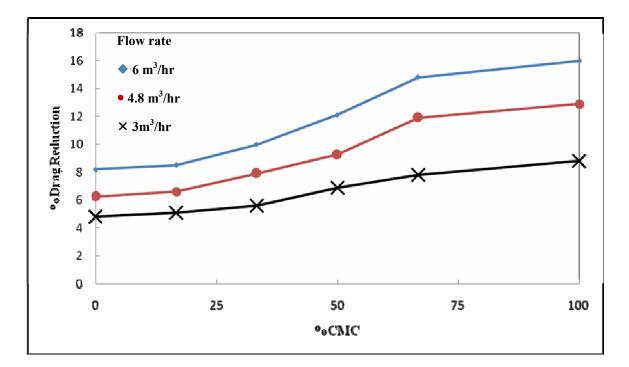
Fig. 4.21 Effect of %CMC mixture with SLS at 300 ppm percentage drag reduction through 1.25 inch I.D pipe.
