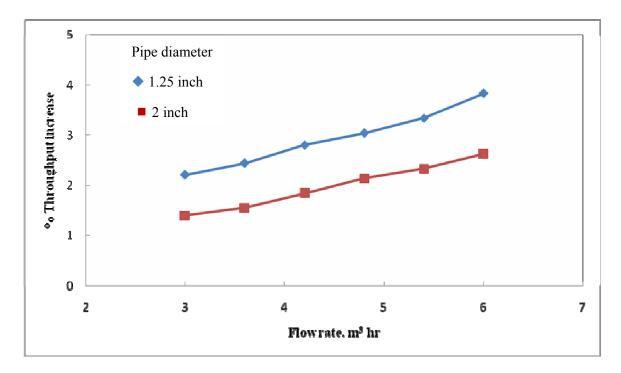
Fig. 4.16 Effect of flow rate on percentage throughput increase for SLS in a 200 ppm.
