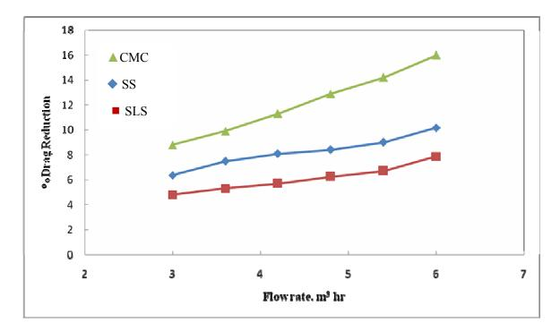
**Fig. 4.18** Effect of flow rate on percentage drag reduction for SS, SLS surfactants and CMC polymer at 300 ppm through 1.25 inch I.D pipe.
