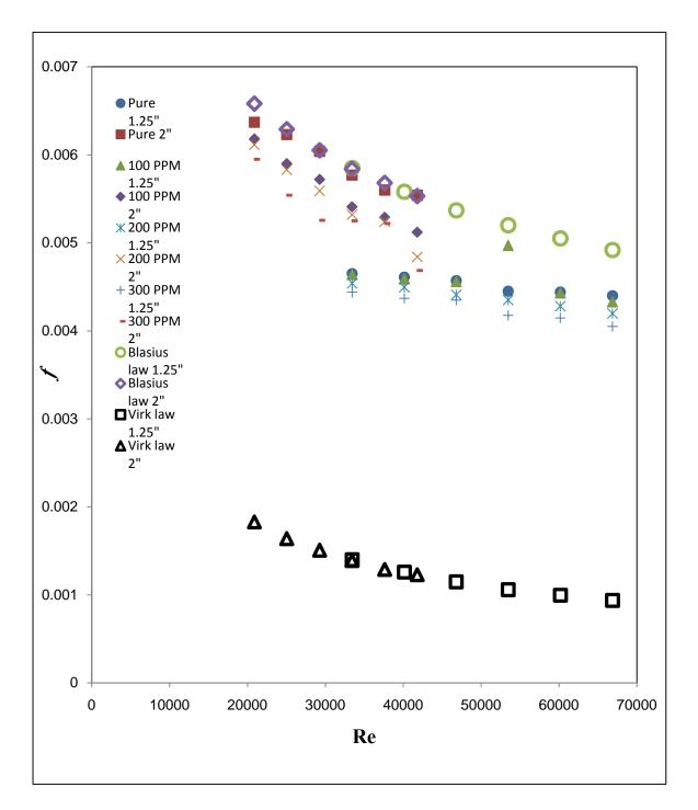
Fig. 4.37 Friction factor as function of Reynolds number for SLS.
