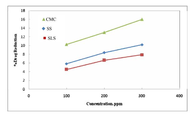
**Fig. 4.17** Effect of concentration on percentage drag reduction for SS , SLS surfactants and CMC polymer at 6.0 m<sup>3</sup>/hr through 1.25 inch I.D pipe.
