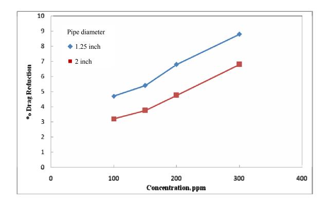
Fig. 4.1 Effect of concentration on percentage drag reduction for CMC of  $3 \text{ m}^3/\text{hr}$ .
