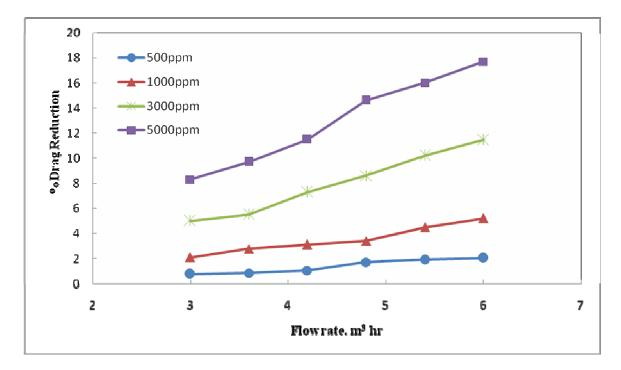
**Fig. 4.28** Effect of flow rate on percentage drag reduction for transported water with clay as suspended solid through 2inch.
