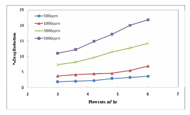
**Fig. 4.27** Effect of flow rate on percentage drag reduction for transported water with clay as suspended solid through 1.25inch.
