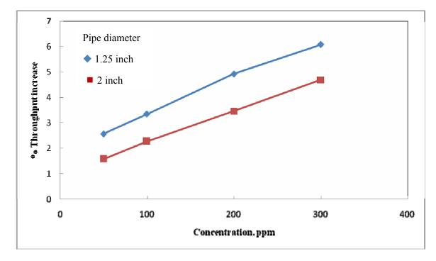
Fig. 4.11 Effect of concentration on percentage throughput increase for SS at  $6m^3/hr$ .
