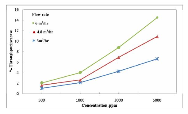
**Fig. 4.25** Effect of concentration on percentage throughput increase for transported water with clay as suspended through 1.25 inch.
