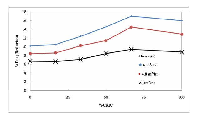
Fig. 4.20 Effect of %CMC mixture with SS at 300 ppm percentage drag reduction through 1.25 inch I.D pipe.
