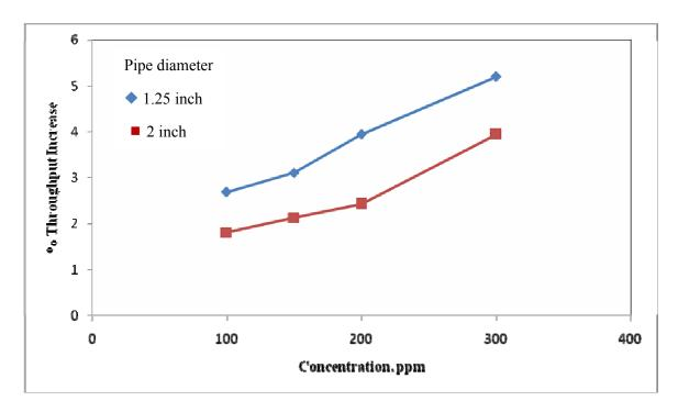
Fig. 4.4 Effect of concentration on percentage throughput increase for CMC of 3  $$m^3/hr$$  .
