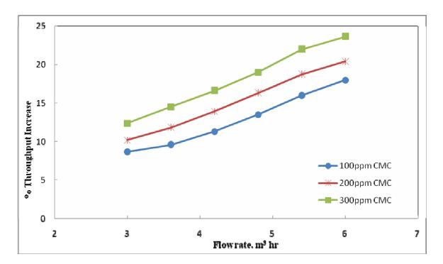
**Fig. 4.33** Effect of adding CMC on percentage throughput increase for water – clay suspension with solid concentration of 5000ppm through 1.25inch I.D pipe
