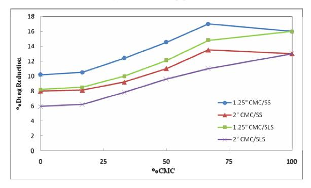
**Fig. 4.22** Effect of %CMC mixture with surfactant at 300 ppm on percentage drag reduction for two pipe at 6m<sup>3</sup>/hr.
