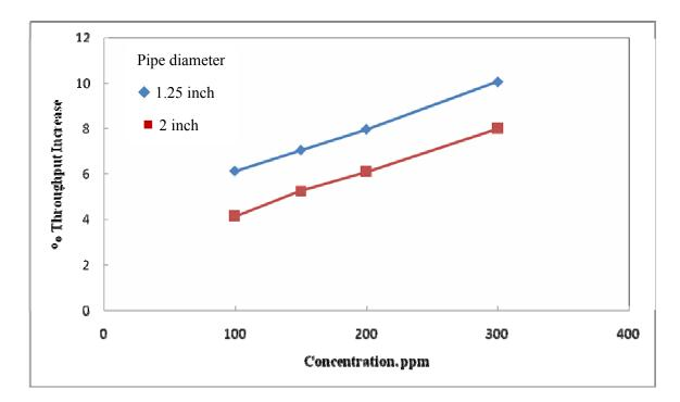
Fig. 4.5 Effect of concentration on percentage throughput increase for CMC at 6  $m^3/hr$ .
