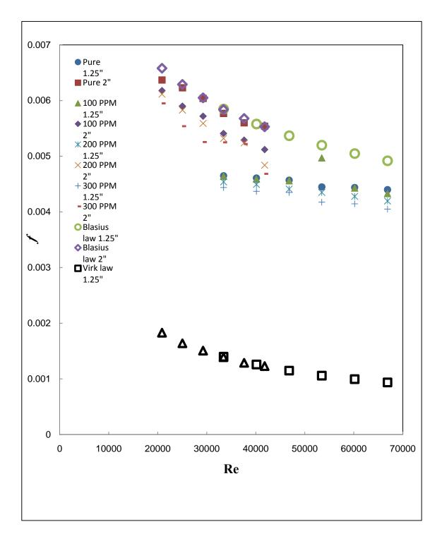
Fig. 4.35 Friction factor as function of Reynolds number for CMC.
