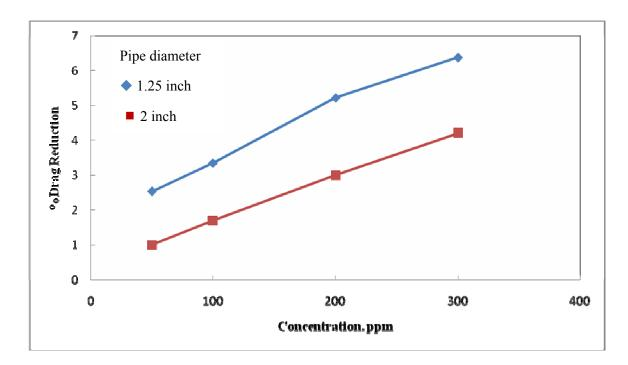
Fig. 4.7 Effect of concentration on percentage drag reduction for SS at 3m<sup>3</sup>/hr.
