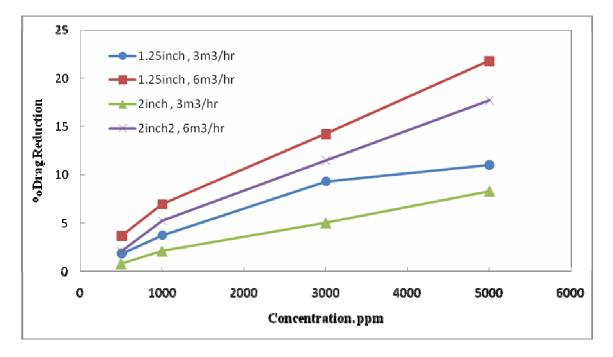
**Fig. 4.29** Effect of pipe diameter on percentage drag reduction with different concentration of clay.
