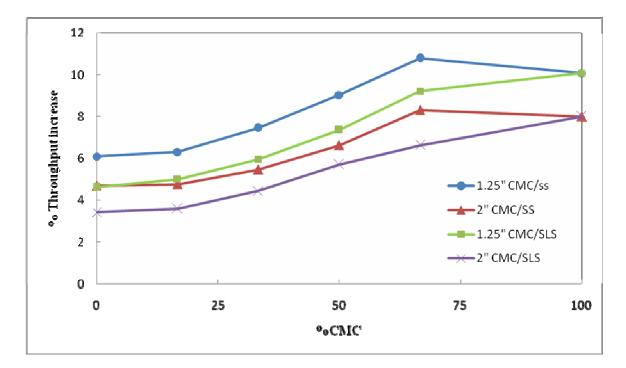
**Fig. 4.23** Effect of %CMC mixture with surfactants at 300ppm on percentage throughput increase for two pipe at 6m<sup>3</sup>/hr.
