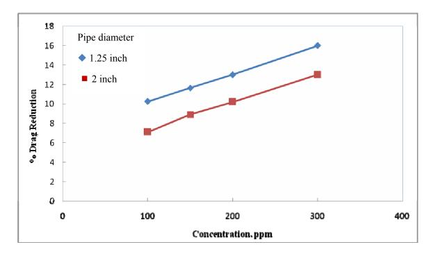
Fig. 4.2 Effect of concentration on percentage drag reduction for CMC at  $6 \text{ m}^3/\text{hr}$ .
