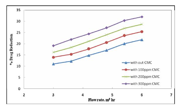
Fig. 4.30 Effect of adding CMC on percentage drag reduction for water – clay suspension with solid concentration of 5000ppm through 1.25inch I.D pipe
