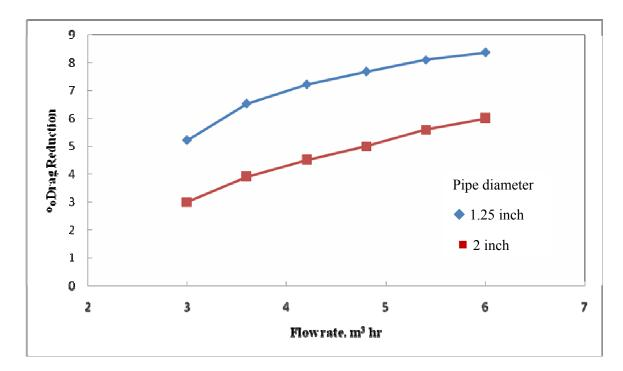
Fig. 4.13 Effect of flow rate on percentage drag reduction for SS in a 200 ppm.
