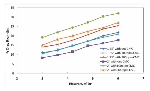
Fig. 4.32 Effect of pipe diameter on effectiveness of CMC/clay additive as drag – reducer/ 5000ppm clay
