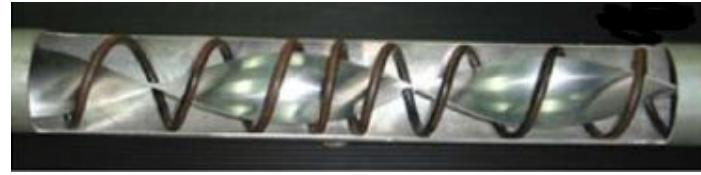
**Figure 2-1:** Compound wire coil/ twisted tape insert tested by Eiamsa-ard et al [11].
