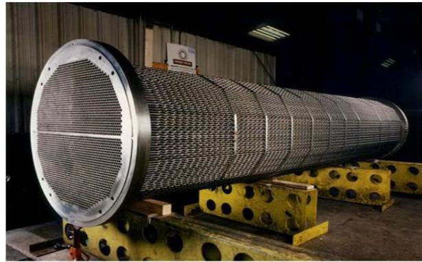
**Figure 2-8:** Completed twisted tube bundle [26].
