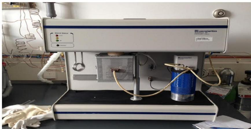
Figure ( 2-7): Micromeritics AutoChem HP Chemisorption Analyzer (BET) (Karlsruhe Institute of Technology, Germany).
