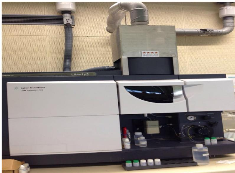
Figure (2-9): Inductively Coupled Plasma - Atomic Emission Spectrometry (Karlsruhe Institute of Technology, Germany).
