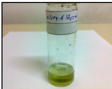
Picture (3.12):- Olive green colored solution for NiSO 4 .6H 2 O in hydrated ammonium aluminum sulfate/urea room temperature ionic liquid with added KSCN 1:30 mole ratio respectively.
