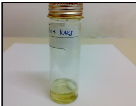
Picture (3.11):- Green colored solution for NiSO 4 .6H 2 O in hydrated ammonium aluminum sulfate/urea room temperature ionic liquid with added KSCN 1:10 mole ratio respectively.
