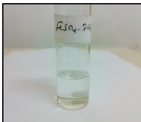
Picture (3.4):- 0.03 M colorless solution for \text{FeSO}_4 \cdot 7\text{H}_2\text{O} in hydrated ammonium aluminum sulfate/urea room temperature ionic liquid dissolved at 40°C.
