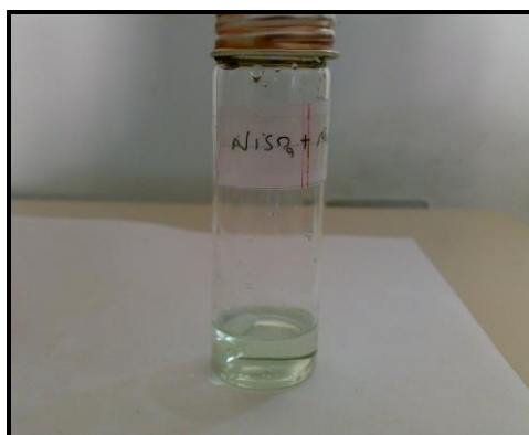
Picture (3.13):- Faint green solution for \text{NiSO}_4 \cdot 6\text{H}_2\text{O} in hydrated ammonium aluminum sulfate/urea room temperature ionic liquid with addition \text{NaNO}_2 1:1 mole ratio respectively.
