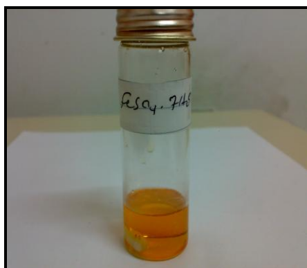
Picture (3.5):- Orange colored solution for \text{FeSO}_4 \cdot 7\text{H}_2\text{O} in hydrated ammonium aluminum sulfate/urea ionic liquid with addition KSCN 1:1 mole ratio dissolved at 40^\circ\text{C} .
