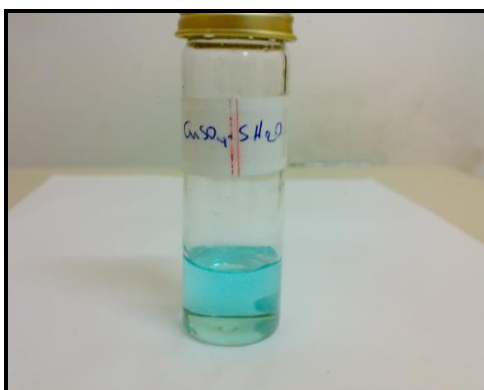
Picture (3.14):- 0.05 M blue colored solution for \text{CuSO}_4 \cdot 5\text{H}_2\text{O} in hydrated ammonium aluminum sulfate/urea room temperature ionic liquid dissolved at 40°C.
