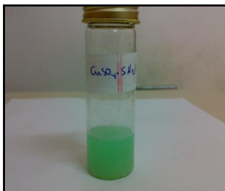
Picture (3.15):- Green colored solution for \text{CuSO}_4 \cdot 5\text{H}_2\text{O} in hydrated ammonium aluminum sulfate/urea room temperature ionic liquid with addition KSCN (1:0.25) mole respectively.
