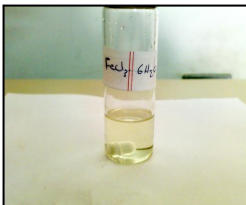
Picture (3.2):- 0.01 M pale yellow solution for \text{FeCl}_3 \cdot 6\text{H}_2\text{O} in hydrated ammonium aluminum sulfate/urea room temperature ionic liquid dissolved at 40°C.
