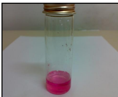
Picture (3.7):- 0.05 M of pink colored solution for \text{CoSO}_4 \cdot 7\text{H}_2\text{O} in hydrated ammonium aluminum sulfate/urea room temperature ionic liquid dissolved at room temperature.
